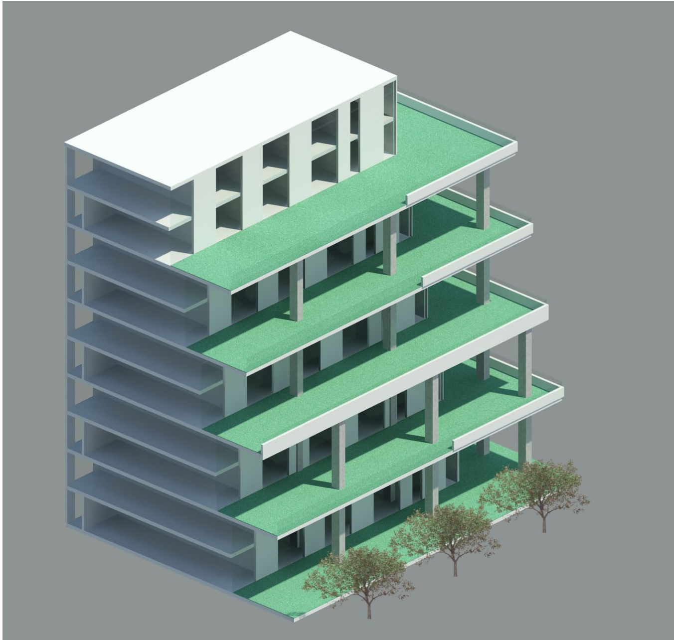
FIG. 4.84 TYPE E - MID RISE STACKED DWELLINGS WITH VERTICALLY WITH SET-BACK AND STACKED TERRACES
