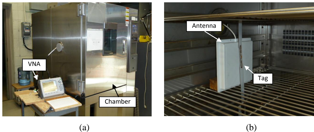
Figure 22: Illustration of experimental setup; (a) environmental chamber and network analyzer; (b) tag and antenna.
