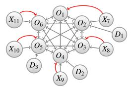
Figure 6.13: The complete graph structure system with six plant agents and three disturbance agents.
