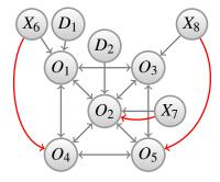
Figure 7.6: The wheel structured nonlinear system with five plant agents and two disturbance agents.
