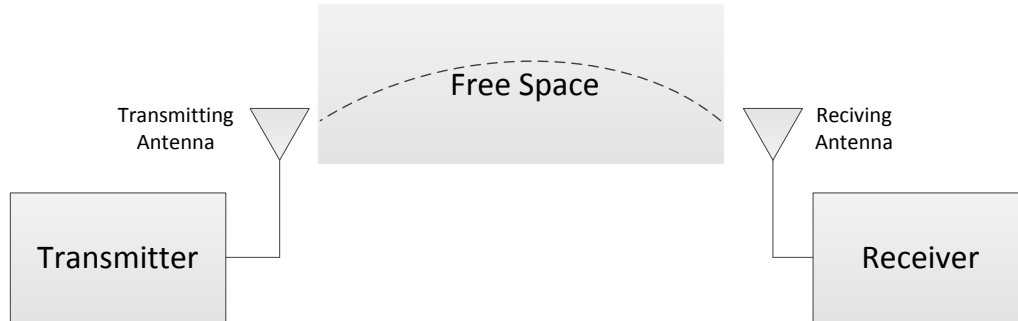
Figure 2.3: Functional blocks of a typical Wireless Power Transfer (WPT) system.
