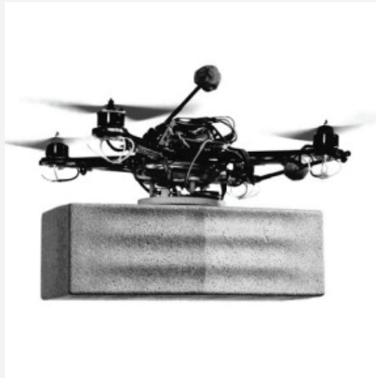
FIG 61 Drone lifting a polystyrene block.
