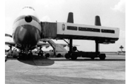
[1.64] A view of a fully-raised jetway extended to meet a plane for easy passenger boarding, c. 1970's.
