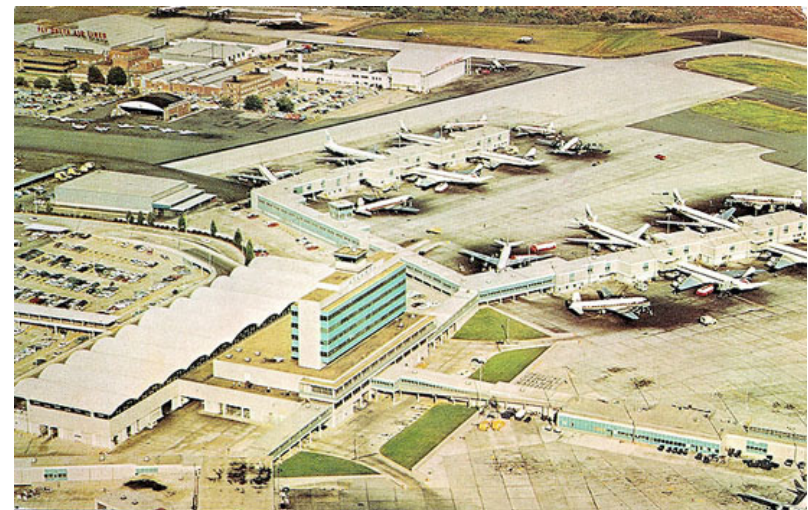
[1.59] An aerial photograph of Hartsfield Atlanta Airport showing its multi-pier finger design, 1961.
