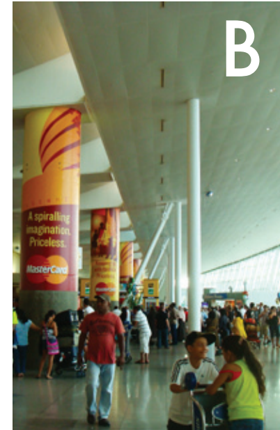
[2.42] Very public arrivals hall at JFK T4. A poor layout that emphasizes sideways circulation leads to congestion.
