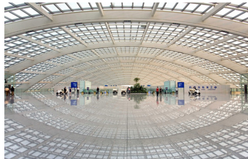
[1.1.49] The Ground Transportation Centre (or GTC) at Beijing Capital Airport. The space is made to feel larger than it actually is through the use of highly-reflective, polished stone flooring.
