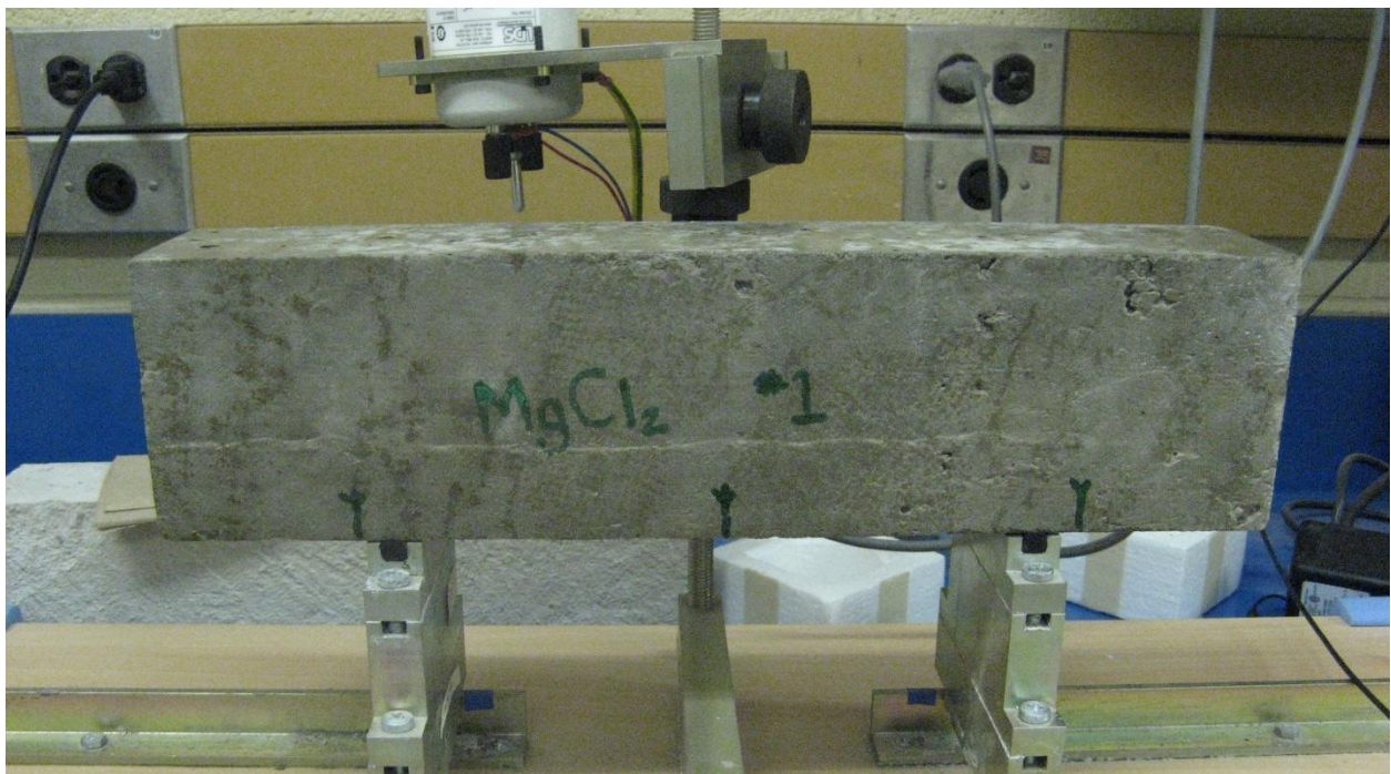
Figure 5.1-3 - MgCl 2 freeze and thaw prism number one front after 385 freeze and thaw cycles
