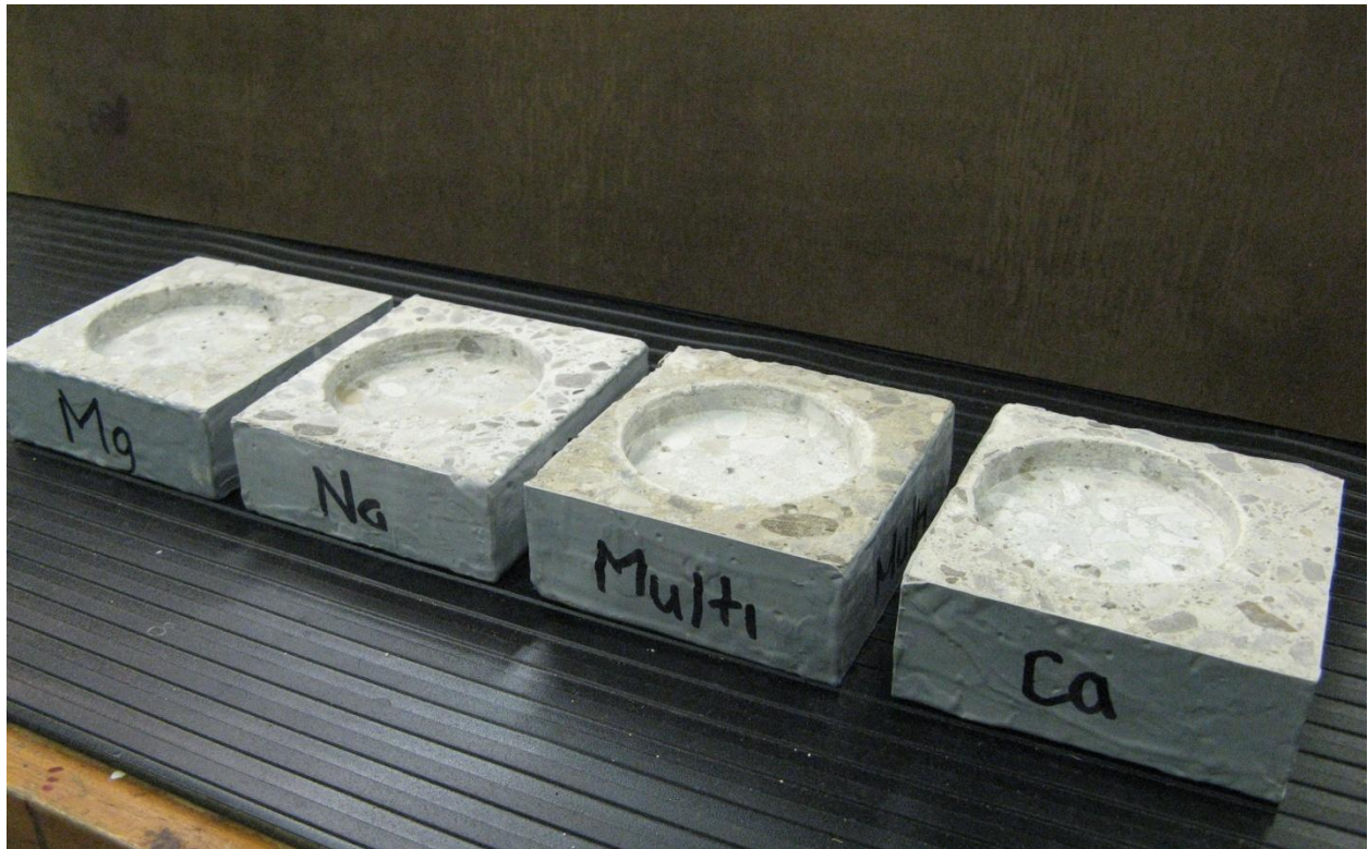
Figure 3.2-11 - Post-grinding chloride penetration samples
