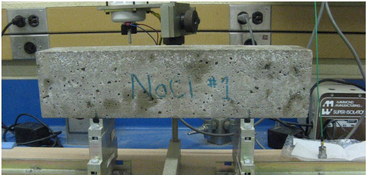
Figure 5.1-5 - freezing and thawing set 2, diluted solutions, NaCl prism one after 355 freezing and thawing cycles
