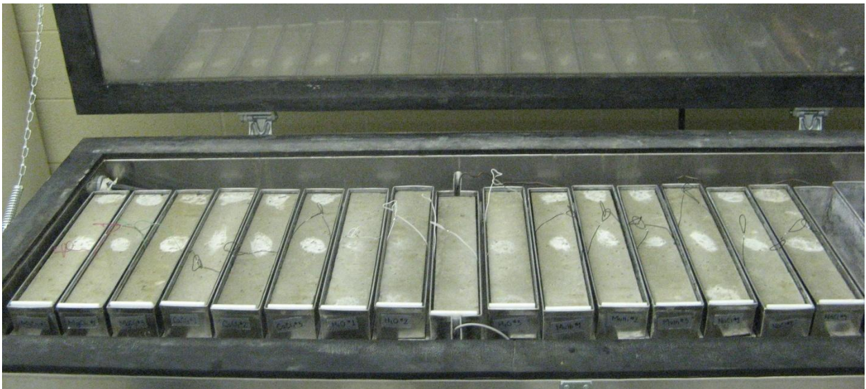
Figure 3.2-1 - Freezing and thawing chamber with lid open, prisms submerged in solution or water
