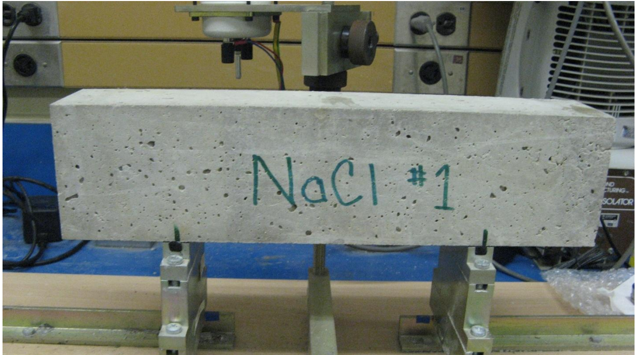
Figure 5.1-4 - freezing and thawing set 2, diluted solutions, NaCl prism one prior to exposure
