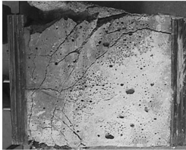
Figure 2.2-2 - Fracture of mortar specimen caused by \text{CaCl}_2 [1]
