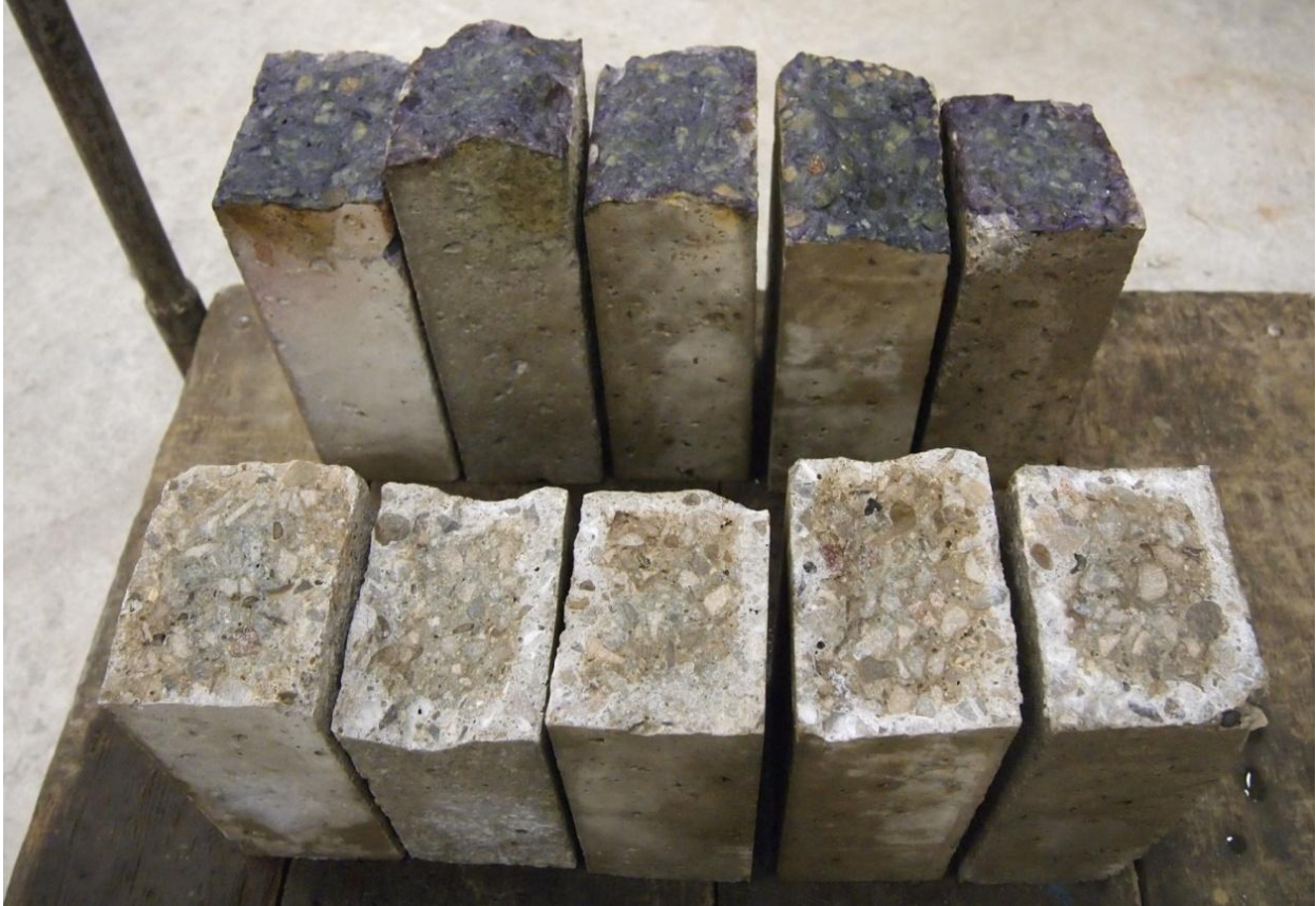
Figure 3.2-12 - pH (top) and \text{AgNO}_3 (bottom) spray indicators on concrete specimens
