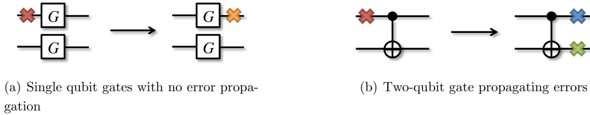
Figure 1.3: Difference in error propagation between one-qubit gates and two-qubit gates within an error correction codeblock.
