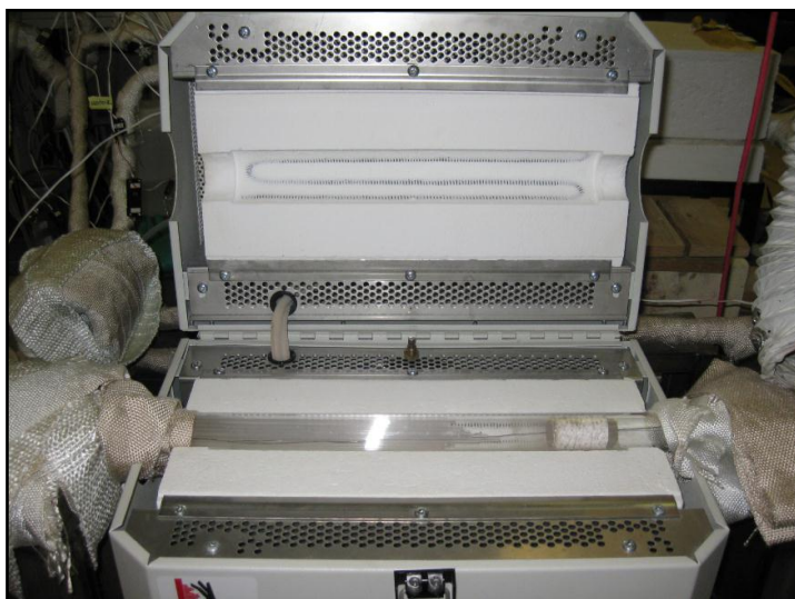
Figure 3-5: Furnace portion of the tube reactor system, with a DOC catalyst inserted.
