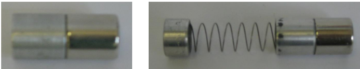
Figure 17 – End magnet assemblies: SDOF (left) and MDOF (right)
