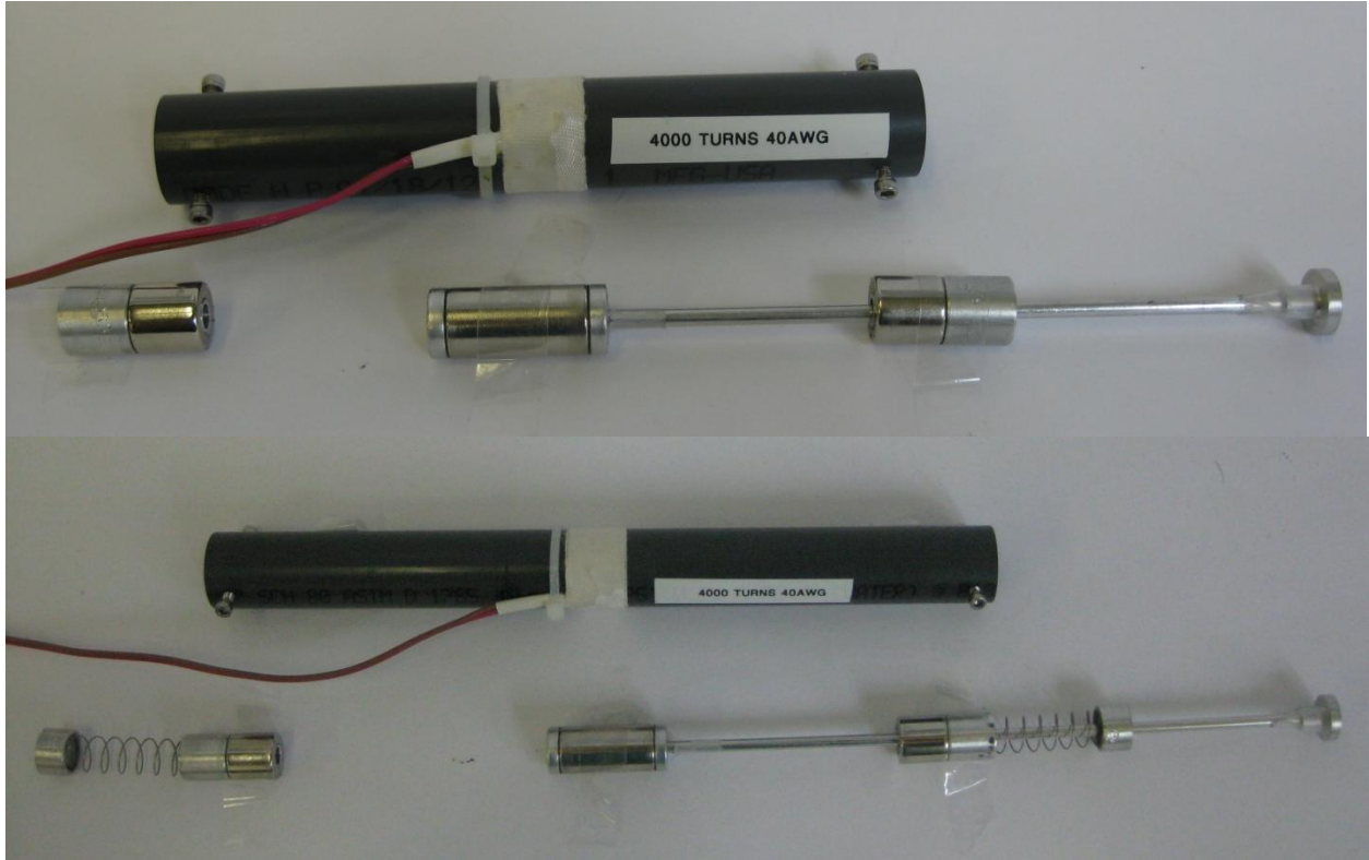
Figure E5 – Exploded view of SDOF (top) and MDOF (bottom) prototypes
