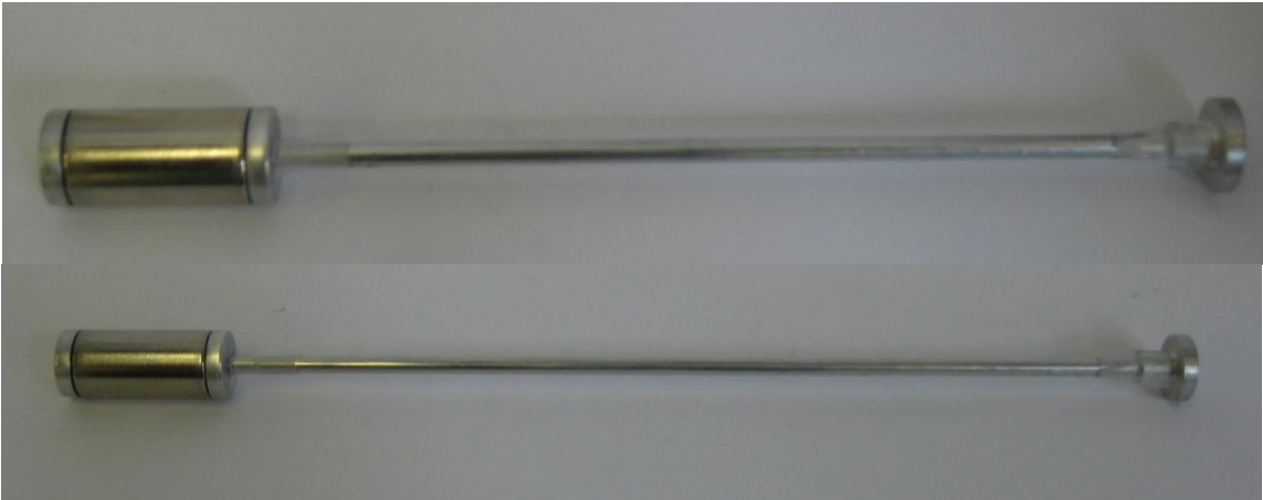
Figure 16 - Middle magnet assemblies: SDOF (top) and MDOF (bottom)
