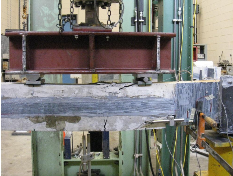
Figure 5.30 Flexural failure of Beam M-350-R-m.
