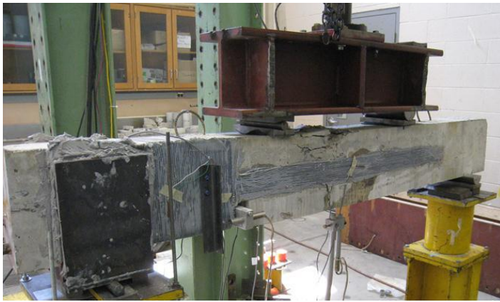
Figure 5.70 Failure of Beam F-350-R-m-140 by concrete crushing.
