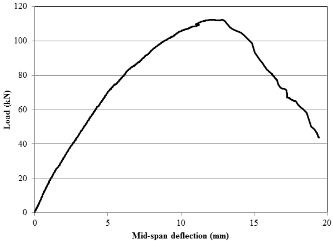
Figure 4.16 Load versus mid-span deflection for Beam M-A-100-5.
