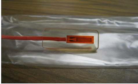
Figure 3.13: Encapsulated strain gauge.
