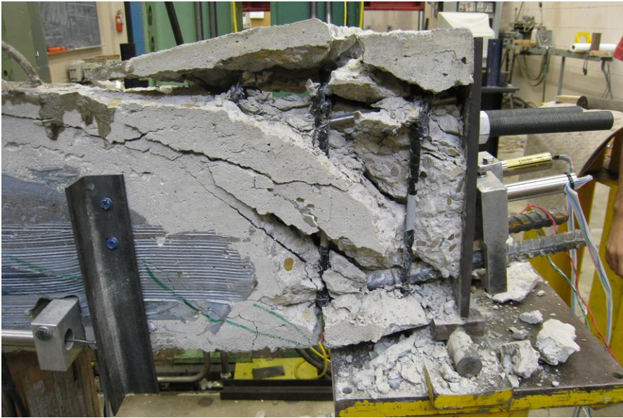
Figure 4.42 The anchorage zone for Beam F-B-97-0 after failure in the testing frame.
