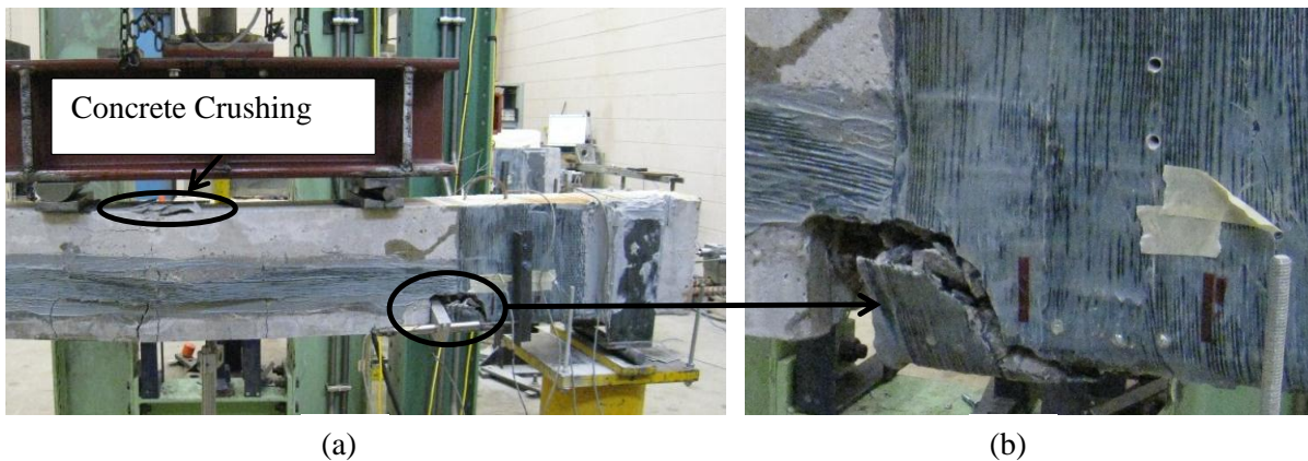
Figure 5.37 Final failure of Beam M-350-R-h by crushing of concrete. Part of the FRP ruptured close to the pocket.
