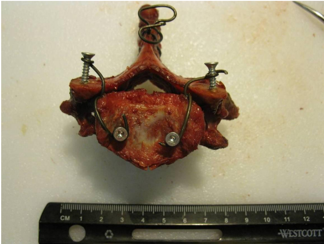
Figure 4-2: C6-C7 Segment Ready for Potting
