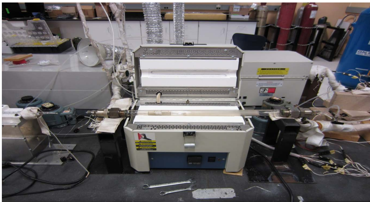
Figure 8: Reactor tube and Lindberg/Blue Mini-Mite tube furnace
