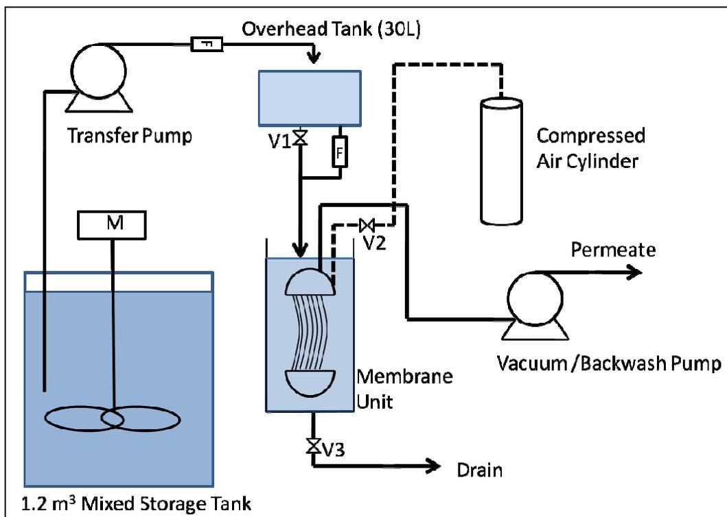
**Figure 4.1: Schematic of Experimental Setup**
