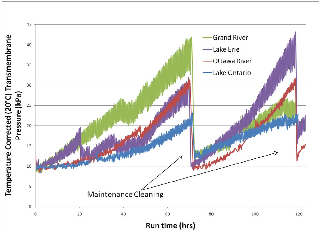
**Figure 4.2: Fouling profile of four waters**
