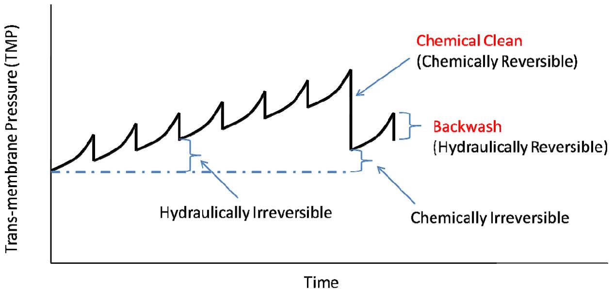
**Figure 2.5: Fouling components during constant flux LPM filtration**
