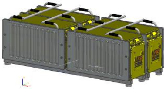
Figure 24: Battery Modules with Cold Plates on all Side Thermal Surfaces
