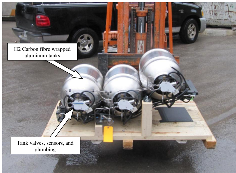
Figure 31: GM/Quantum Hydrogen Storage System
