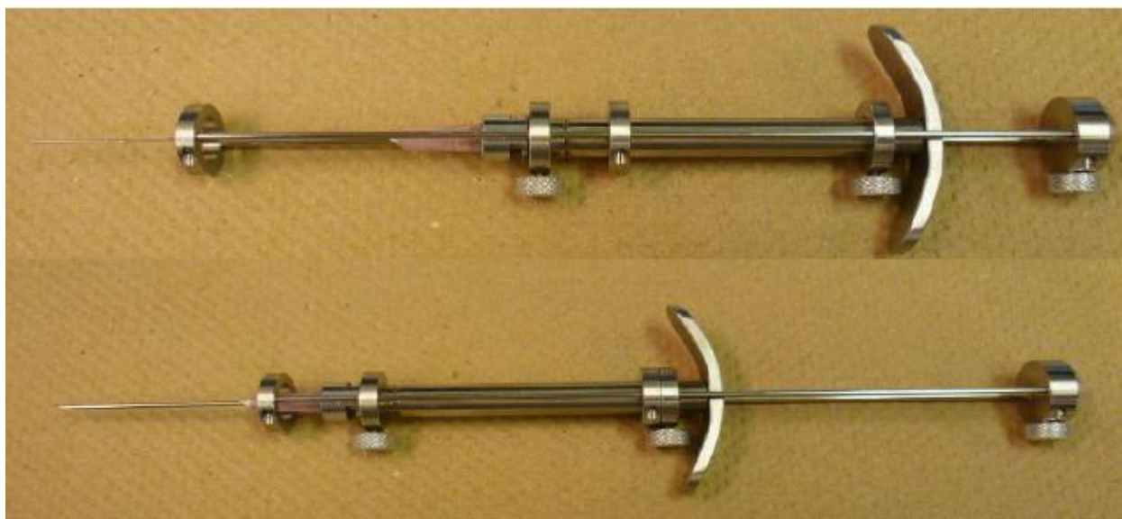
Figure 6:1 Schematic diagram of in vivo tissue sampling device (above). In vivo SPME device with PDMS biocompatible coating (Top) Depressing the plunger exposes 1.5 cm SPME coating during the extraction. (Bottom) The device is shown retracted for storage. (University of Waterloo machine shop made this device for us)
