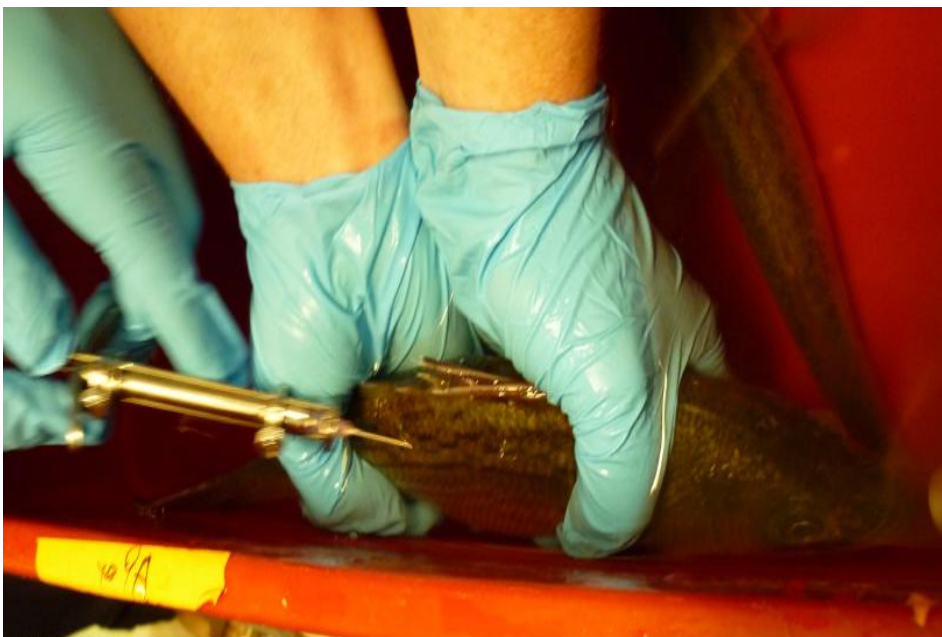
Figure 6:2 In vivo SPME device being used for sampling pharmaceuticals in live fish
