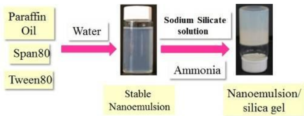
Figure 5.2: Preparation of the nanoemulsion/silica hydrogel.
