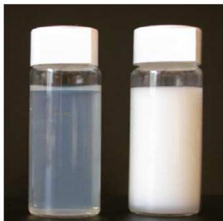
Figure 2.5: Photograph of a nanoemulsion (left) and a macroemulsion (right) with droplet diameters of 35 nm and 1 \mu m, respectively, Reprinted with permission from Ref (48).
