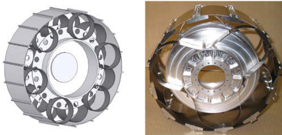
Figure 5.1: Flexible metal wheel used in ExoMars (Patel et al. 2010)
