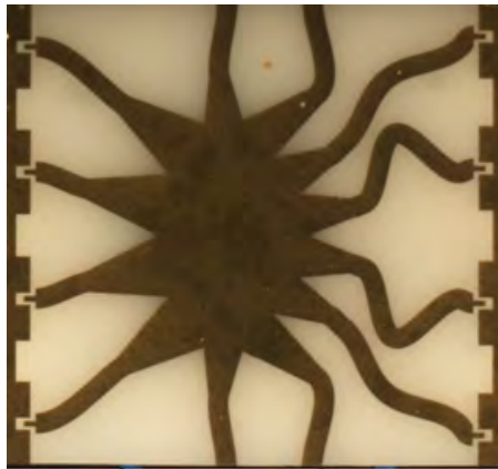
Figure 5.8: Photo of the fabricated 77 GHz Rotman lens on Alumina substrate.
