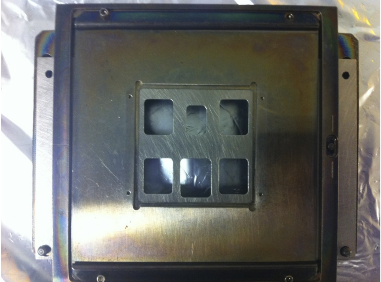
Figure 2.4: Designed mask for cathode deposition mounted onto the sample holder
