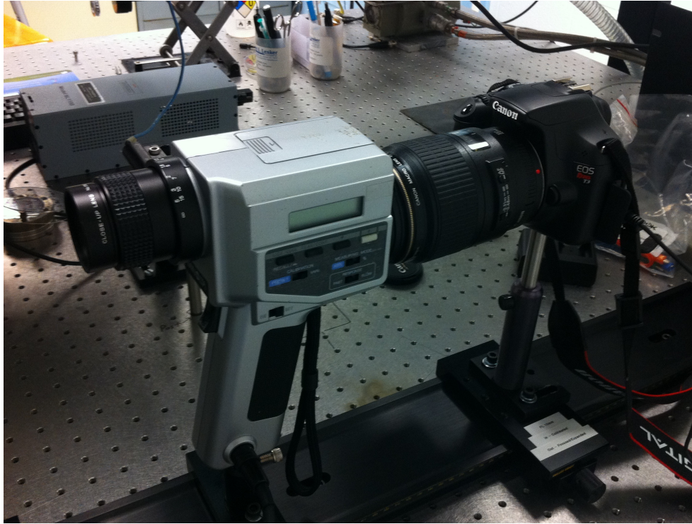
Figure 3.7: The camera system used in our measurement system of imaging upconversion devices
