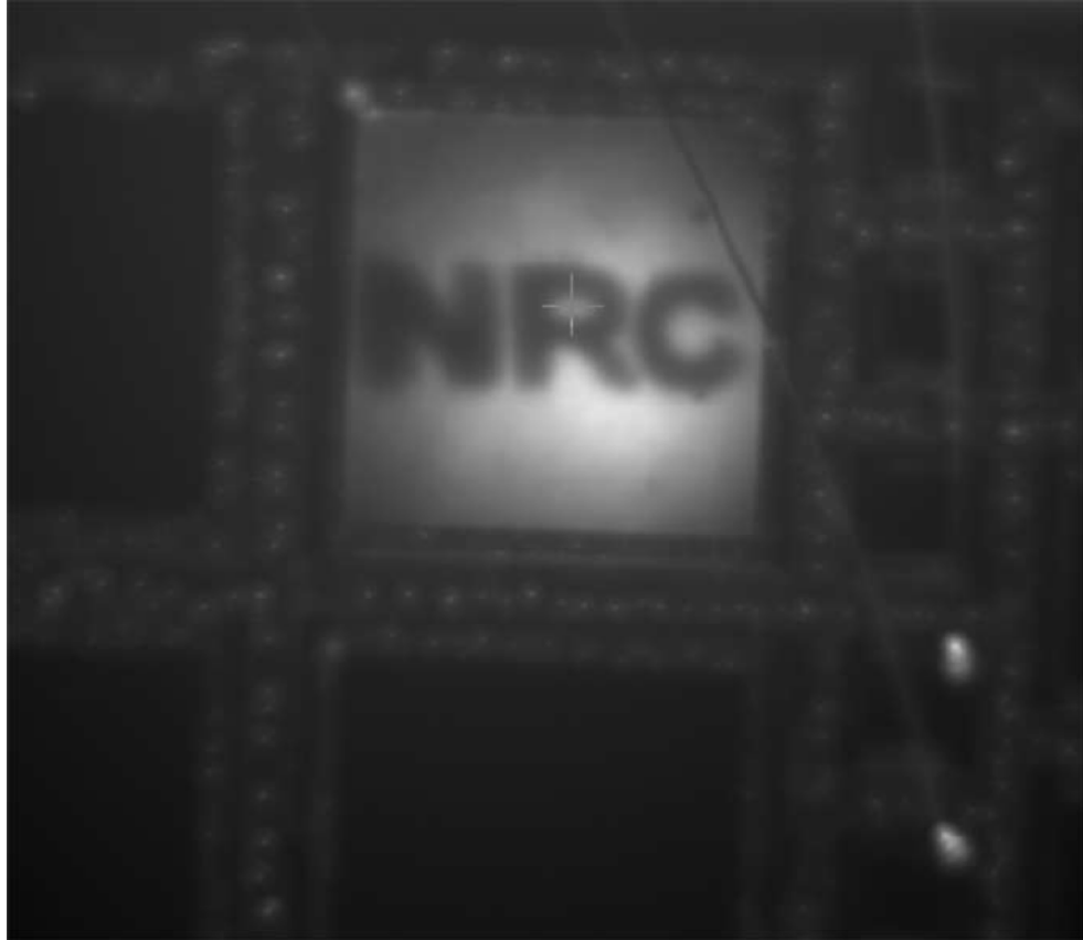
Figure 1.12: CCD imaging of letters "NRC" obtained from Luo's pixelless imaging up-conversion device. The device is 1.5 \times 1.5 \text{mm}^2 in size. The device was biased at -3 V at room temperature.[46]
