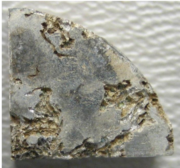
Figure 57: Surface of a corroded Mg-2Ca sample (without Ag deposition) after 168 hours of immersion
