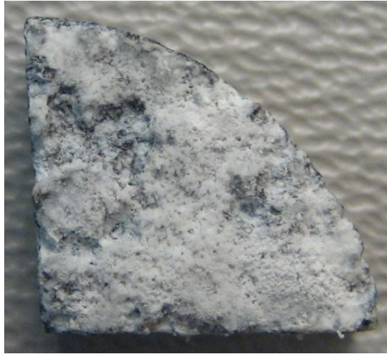
Figure 62: White corrosion products on the surface of an as-cast Mg-2Ca sample after 336 hours of immersion
