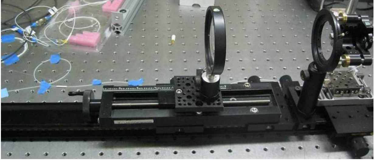
Figure 2.4: A lens mounted on a translation stage allows for control of the loss in the quantum channel by manipulation of the beam size. To the right, upconverted green photons exit a coupler to the single mode fiber carrying the output beam. The quantum receiver is located further away to the left.
