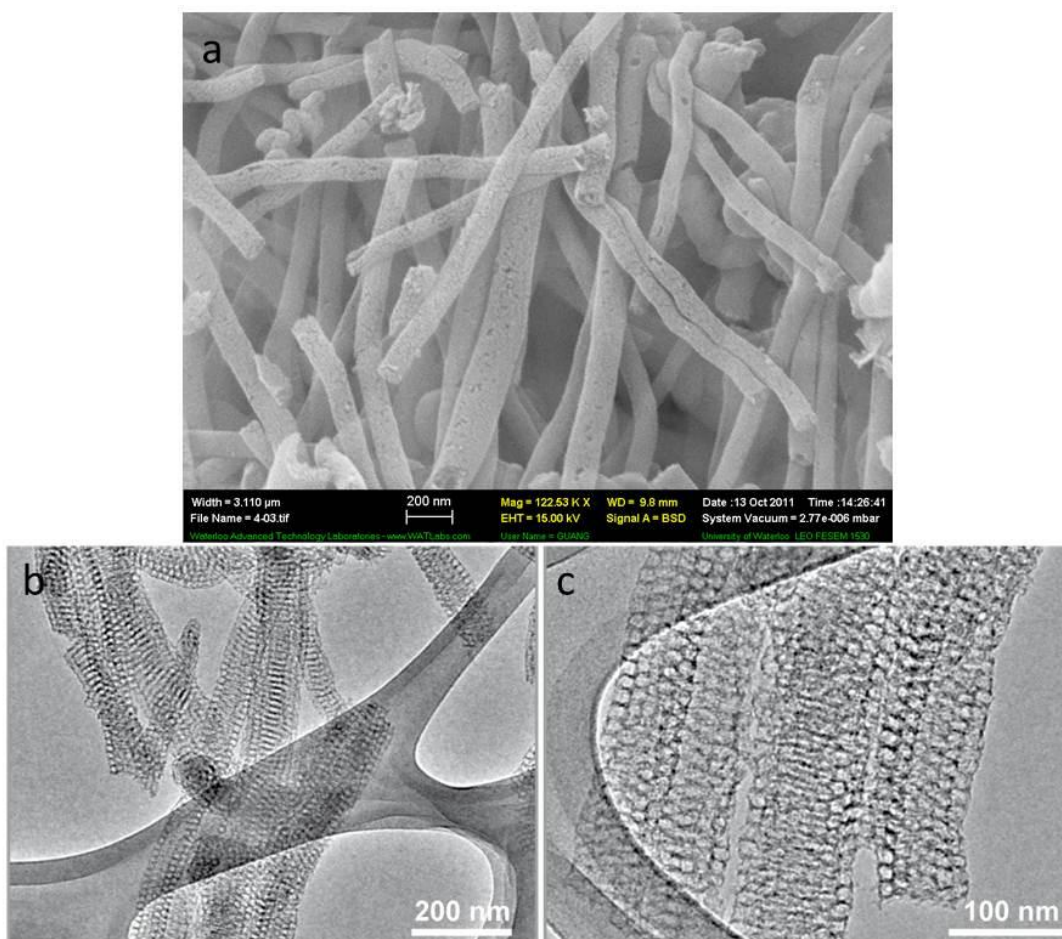
Figure 4.11 (a) SEM and (b, c) TEM images of the mesoporous carbon nanofibers.
