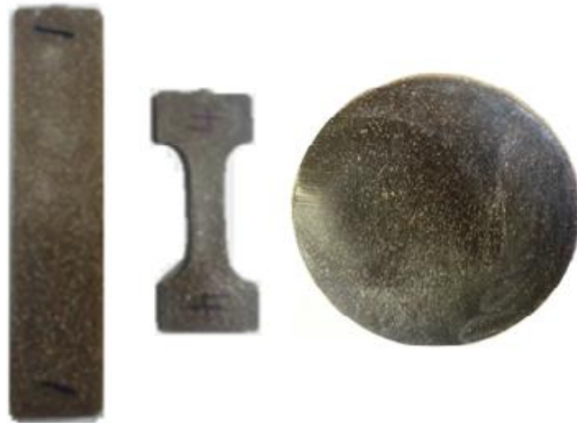
Figure 3.3 Flexural (left, rectangular), Tensile (centre, dumbbell) and Gardner Impact (right, circular) Specimens for Characterizations and Testing
