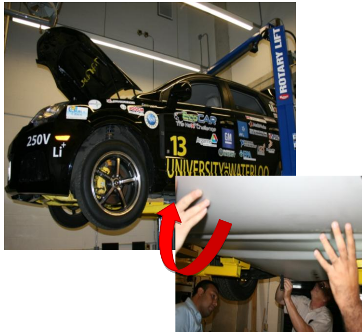
Figure 2.5 The belly pan of a hybrid-electric experimental vehicle will be made from renewable PE
