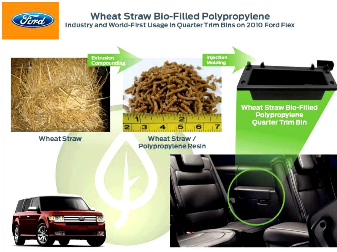
Figure 2.8 Wheat straw-polymer composite as interior part material in Ford Flex 2010
