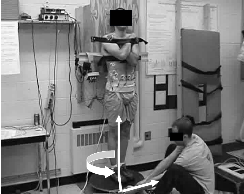
Figure 5.2: To measure twisting stiffness the subject stood on a turntable and the torso was immobilized while a torque was applied to the turntable.
