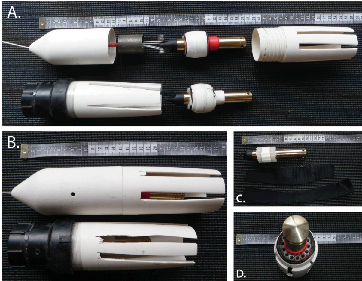
Figure 5.2 Construction of the drag probes. A PVC casing houses a Solinst levellogger thermistor (photo A). 180lb test wire, strung through the tip of the casing, attached to a rope lead, which runs to the boat. The test wire is attached to the cap of the levellogger. Above the cap, weights can be strung on the wire to allow the probe to achieve the desired buoyancy. Slits are cut into the upstream half of the casing, to maximize river flow past the thermistor sensor and to allow debris caught along the sides of the probe to slide out the upstream end. Although the riverbed probe was streamline as much as possible, this was not needed for the river surface probe (photo B). Several layers of material were wrapped around both levelloggers (photo C). The first layer was 0.5cm I.D. polyurethane tubing cut into 5cm lengths. This allowed water movement along the entire length of the probe (photo D). On top of the tubing several layers of neoprene were wrapped, to provide cushioning for the probe as the outside casing scraped along the riverbed.
