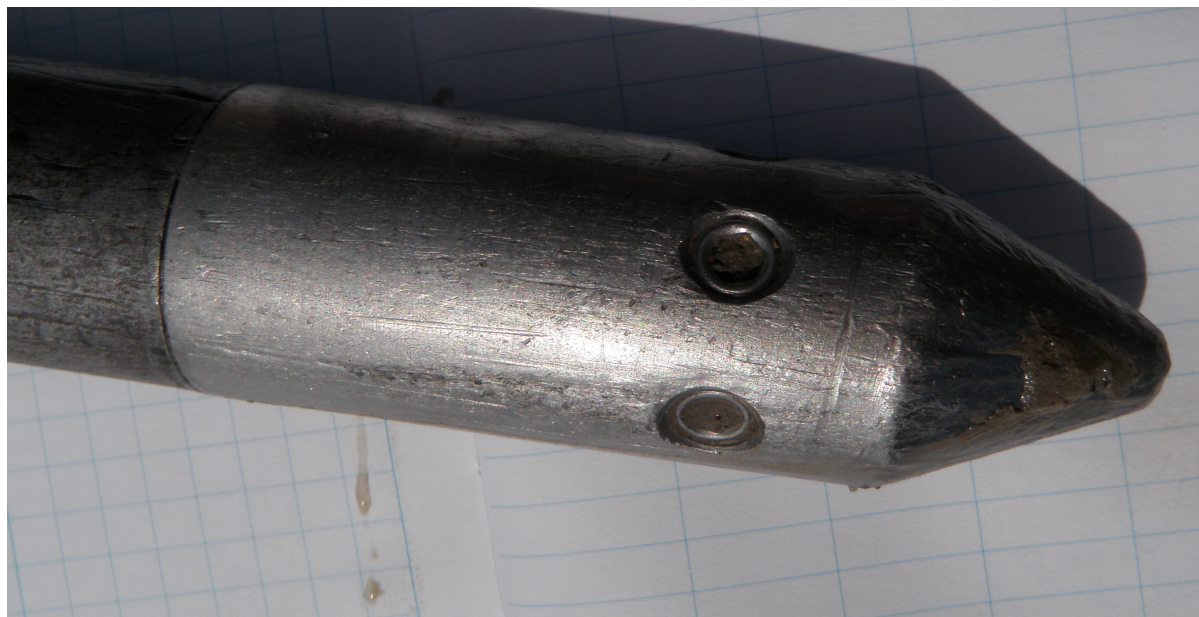
Figure AE.3 Silt clogging the profiler ports at RB-16.
