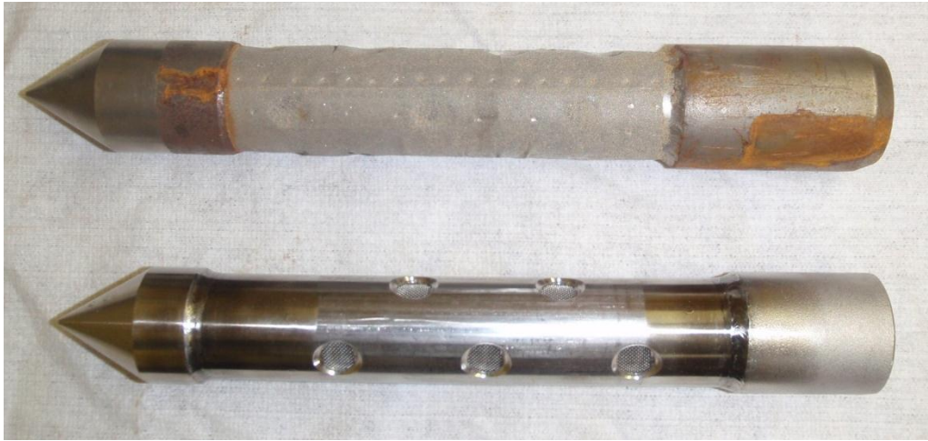
Figure 1.4: The two drive-points used on site. The original drive-point is shown on the bottom (used in locations DP-1 to DP-3), the modified version on top (used in locations DP-4 to DP-6).
