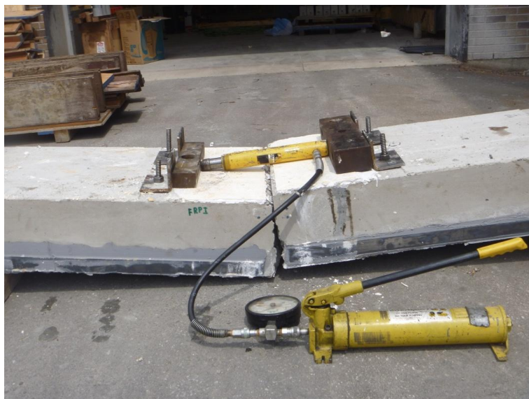
Figure 6-21 – Slab Jacking Arrangement to Separate Slab Halves
