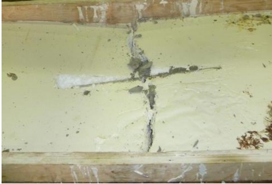
Figure 6-29 –GFRP I-Beam Specimen: GFRP I-Beam Penetration into Geo Foam Layer
