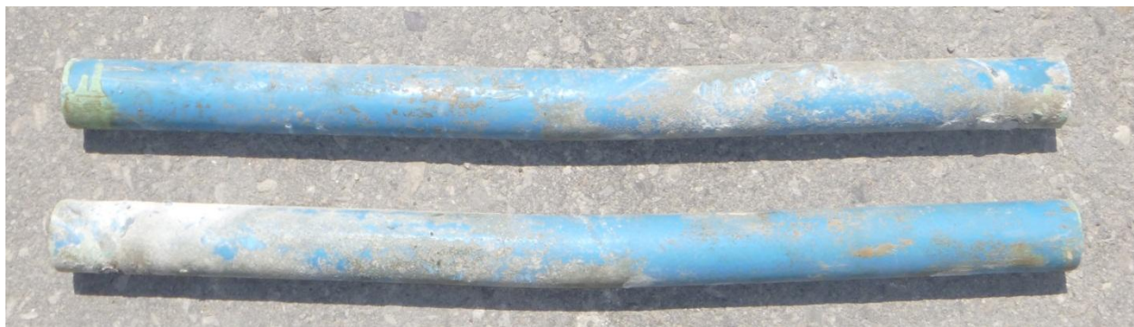
Figure 6-14 – Lab Pilot Dowels after test
