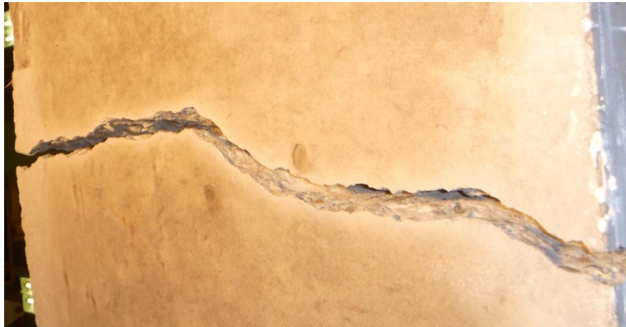
Figure 6-12 – Lab Pilot Bottom of Slab Crack after test
