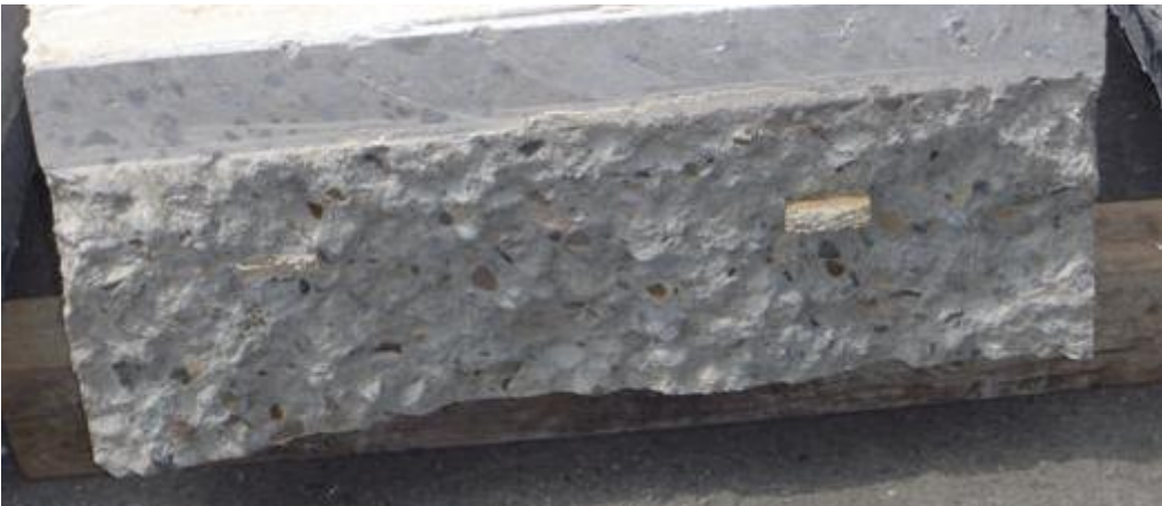
Figure 6-35 - Experimental GFRP Tapered plate Dowel Concrete Joint Faces
