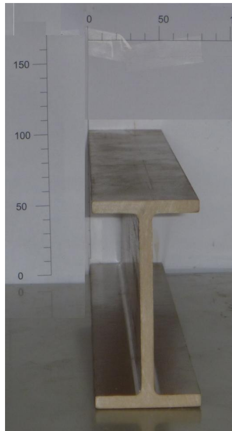
Figure 6-24 – 100 mm x 50mm x 6.4 mm Dynaform GFRP I-beam
