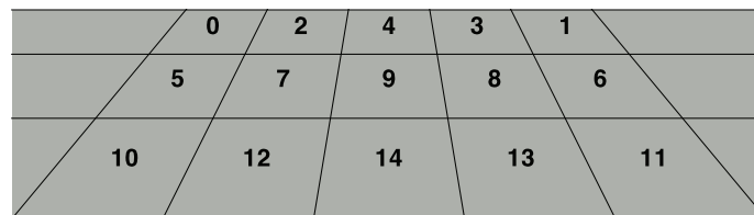
Figure 7.13: A tiled floor with an odd number of tiles along the baseline. To avoid clipping to the quadrant when drawing unit blocks that are along the central vertical, the east and west quadrant tiles are interleaved in a global sequence.
