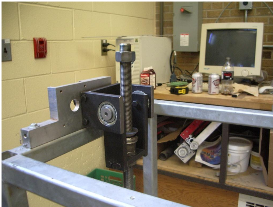
Figure 35: Head Tube Mounting Gimbal, Empty
