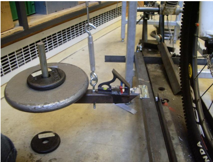
Figure 14: Loading Cage Lever Mechanism
