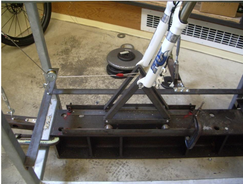
Figure 15: Front Axle Mount and HT MZ Loading Configuration
