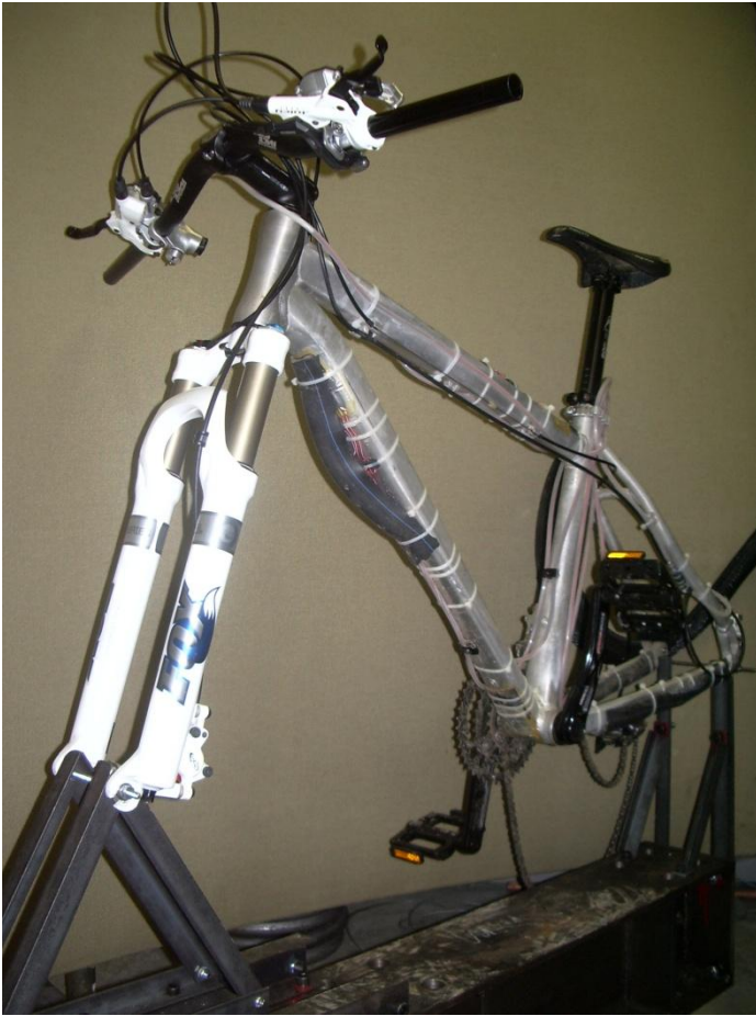
Figure 13: Vertex Frame on Mounting Block Fixture
