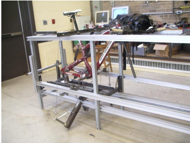
Figure 42: Complete Static Loading Fixture
