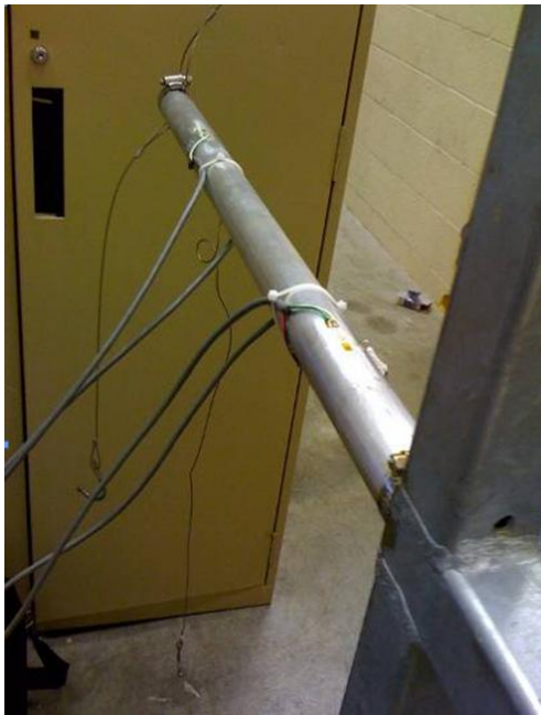
Figure 4: Aluminum Cantilever Beam
