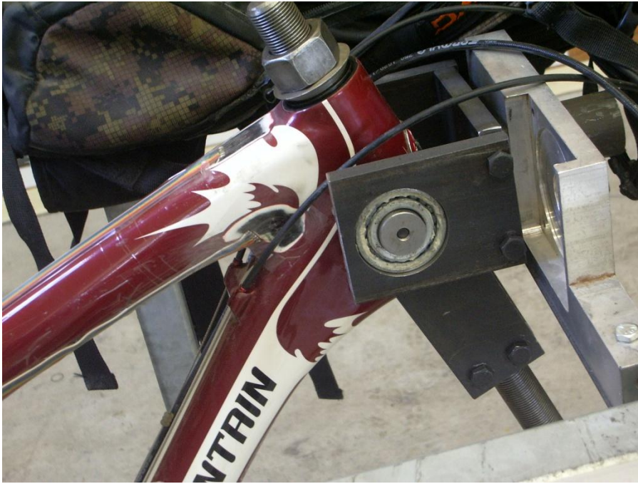
Figure 36: Head Tube Mounting Gimbal, Loaded with Element Frame
