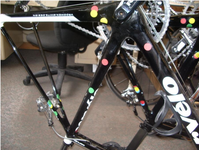
Figure 43: Strain Concentration Locations for Various Loads
