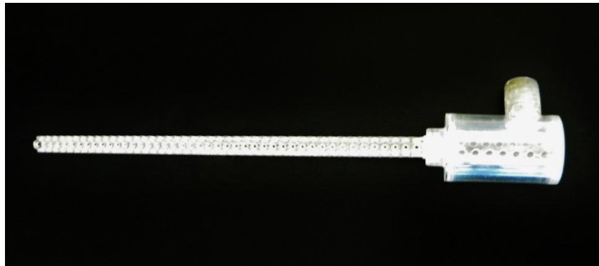
Figure 2.4 Porous manifold to reduce thermal plume – shown horizontally, installed vertically
