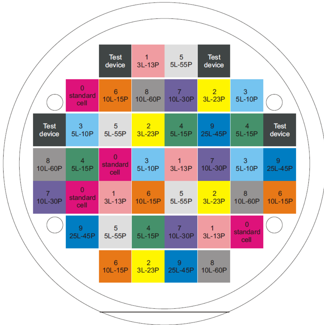
Figure 57 – a color coded map of how different architectures of the designed emitters are spread on the mask. There are 4 instances of each architecture spread uniformly on the wafer to compensate for the random or localized defects over the wafer during processing. the numbers on each square represents the architecture number for the emitter on that area. Table 10 can be used as a reference for each architecture.
