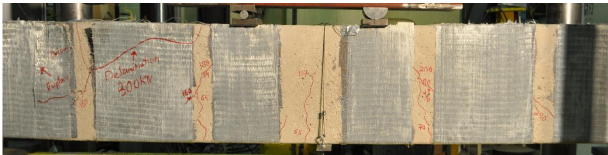
Figure 5-5: Failure of beam 430G-300-NA
