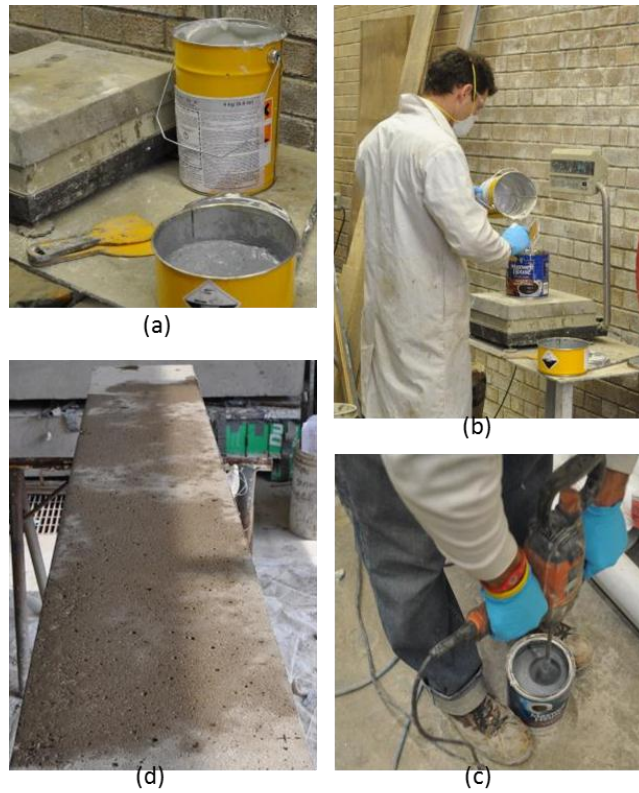
Figure 3-18: Specimen grinding and sandblasting preparation
