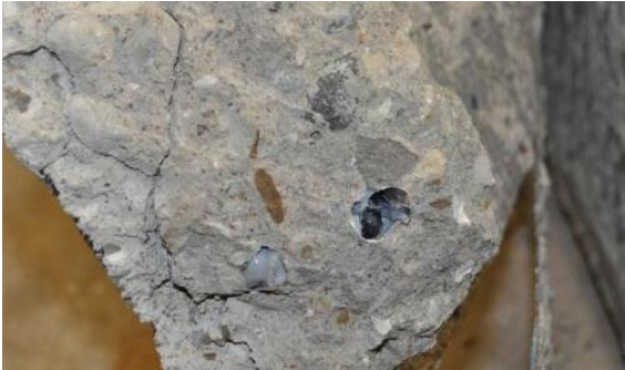
Figure 2-30: FRP anchor pry-out with local concrete failure
