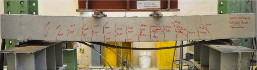
(b) FRP debonding
