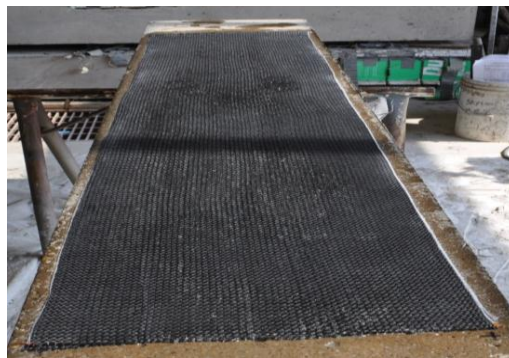
Figure 2-13: Flexural strengthened slab with CFRP sheets
