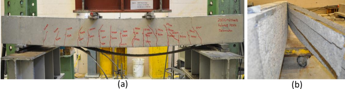
Figure 4-48: FRP debonding failure of slab 230C-2L-NA
