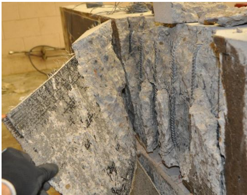
Figure 6-4: Concrete cover failure at steel rebar interface (no anchors)
