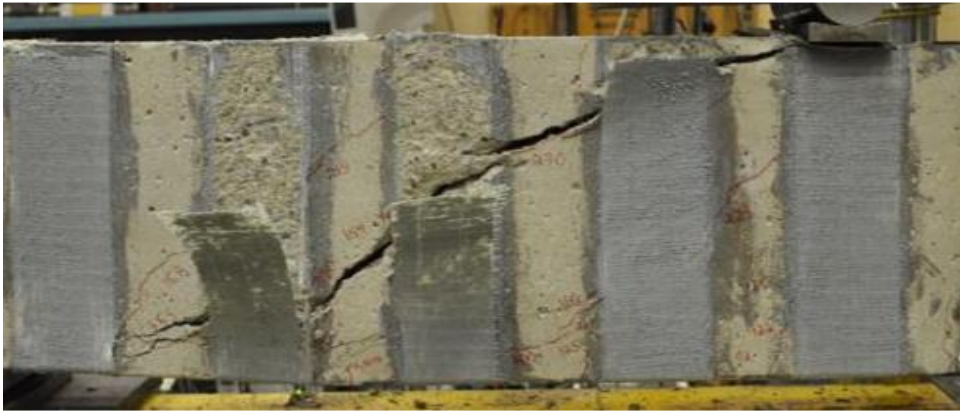
Figure A-15: Failure mode of full depth GFRP strengthened beam (pilot study)
