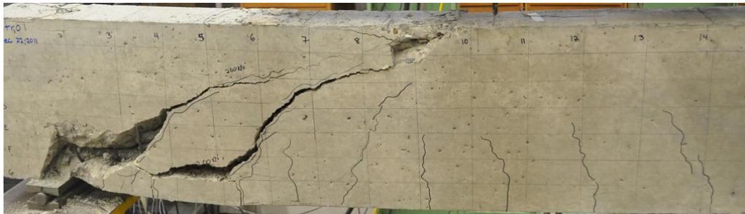
Figure A-1: Failure mode of control beam (pilot study)
