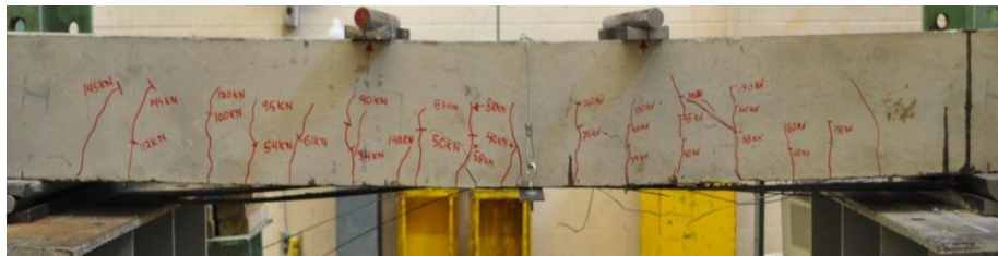
Figure 4-54: FRP debonding of slab 600C-1L-NA
