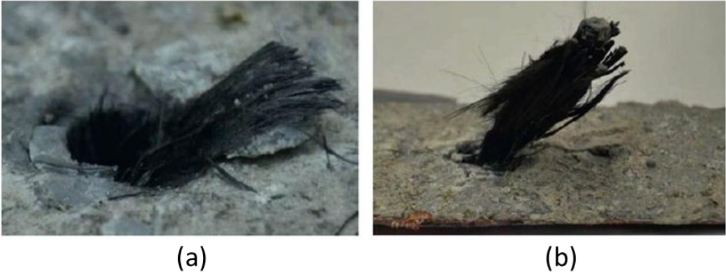
Figure 2-30: FRP anchor pry-out with local concrete failure
