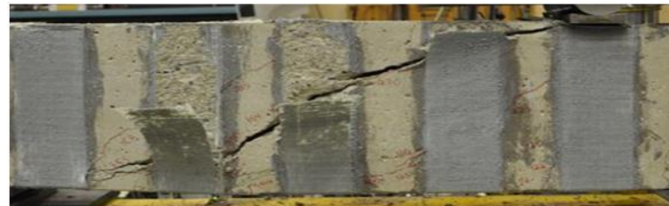
(c) – FRP debonding
