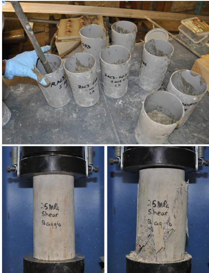
Figure 3-13: Concrete cylinder testing
