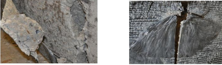
(h) Anchor pullout and rupture
