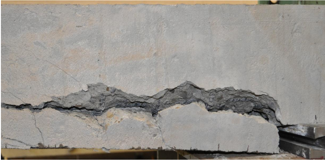
Figure 6-8: Concrete cover failure at concrete/steel rebar interface
