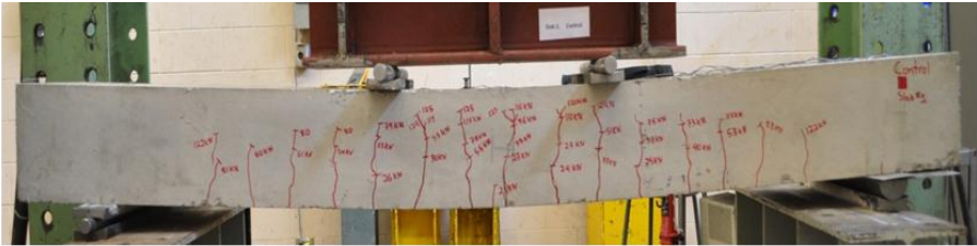
(a) Flexural failure
