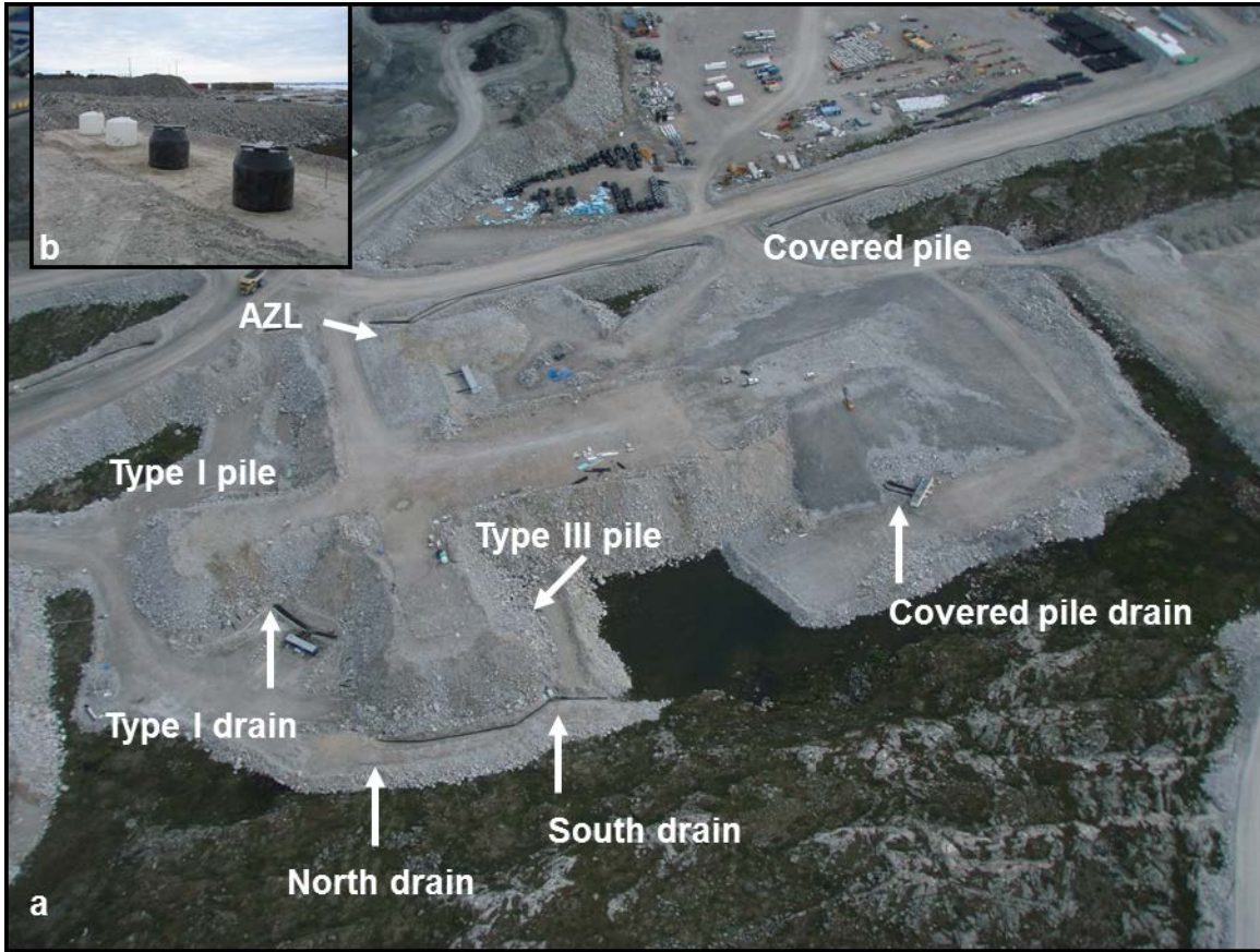
Figure 2.1 Aerial view of the Diavik Waste Rock Research Facility: a) locations of the Type I test pile, Type III test pile, Covered test pile, and AZLs; b) high-density polyethylene barrels used in the construction of the AZLs before rock placement.
