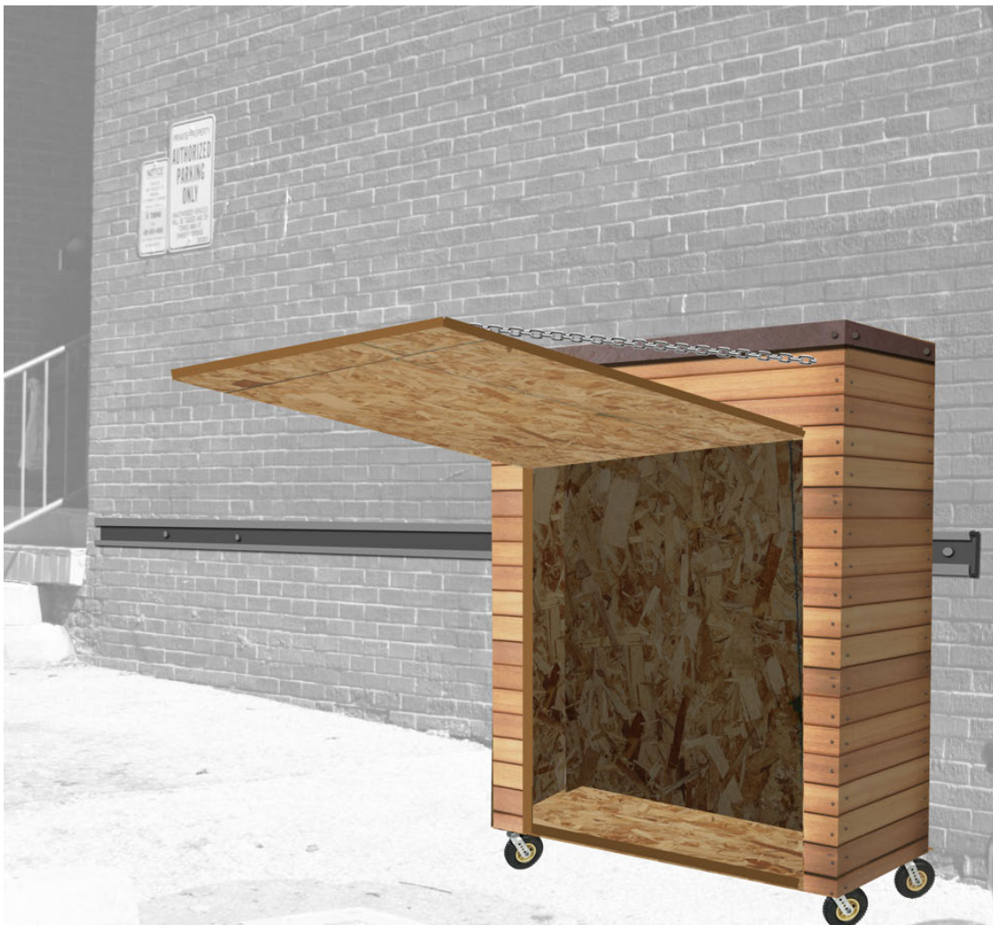
Fig 4.38: A booth locked on the sidewalk storage track.
