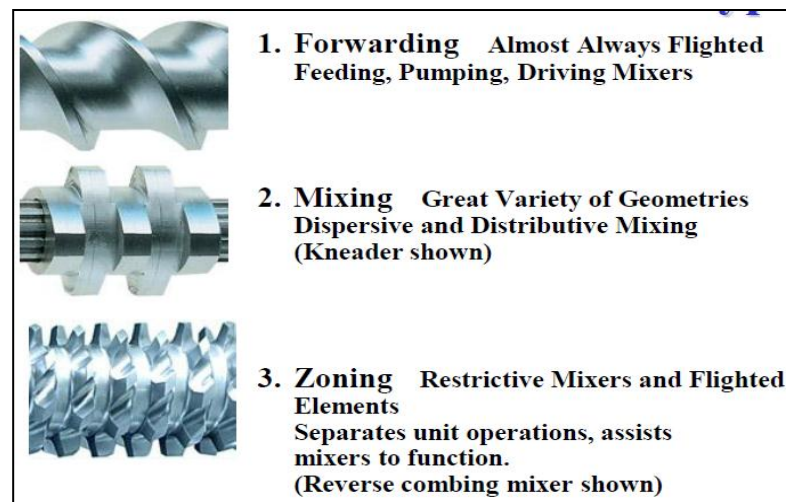
Figure 7.2 Major types of screw elements [2]
