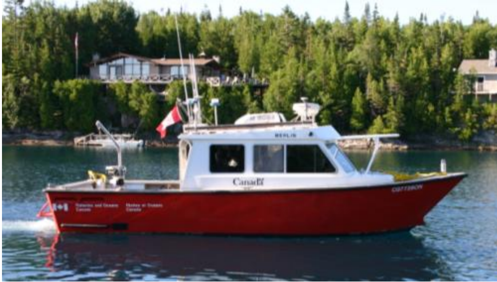
Figure A2.31 CSL Merlin, multibeam sonar launch. Multibeam bathymetric data was collected by the Canadian Hydrographic Service using their survey launch CSL Merlin equipped with a Kongsberg-Simrad EM 3002 multibeam system. The system produced 254 beams spanning an arc of 120 degrees with a ping rate of up to 40 times per second. The swath of lakebed surveyed with each line is 3 to 4 times the water depth. Line spacing is approximately 1.5 times the water depth to provide ensonification overlap between lines. The system is calibrated and all data collected is corrected for roll, pitch, heave and yaw. The differential GPS used for navigation provided an accuracy of +/- 3 m. Survey speed averaged 10 knots resulting in a data collection rate of about 1.2 km 2 /hr in water depth of 40 m with 100% overlap. The raw backscatter data was post-processed by the Geological Survey of Canada and TEKmap Consulting Ltd. In depths less than 10m the resolution is generally 0.5 x 0.5m xy and 1 cm z.
