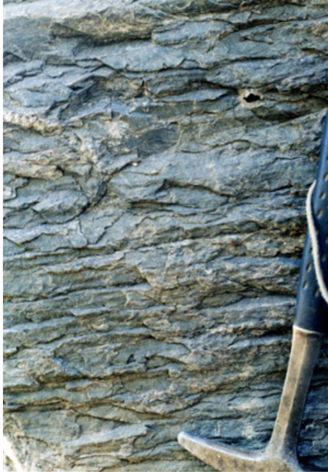
Figure 8-3: Tensile fracture on a tensile joint surface in cordierite hornfels from Iran.
