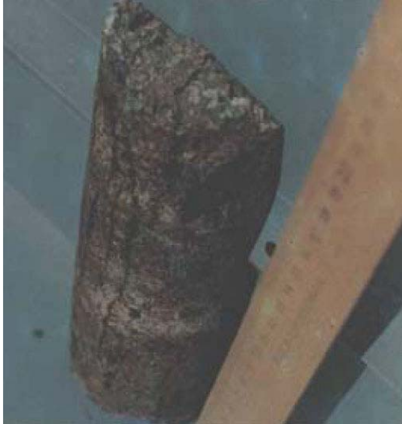
Figure 8-9: Vertical fractures and vugs infilled with heavy oil in a core sample from Kuh-e-Mond field (Photo courtesy of PEDEC).
