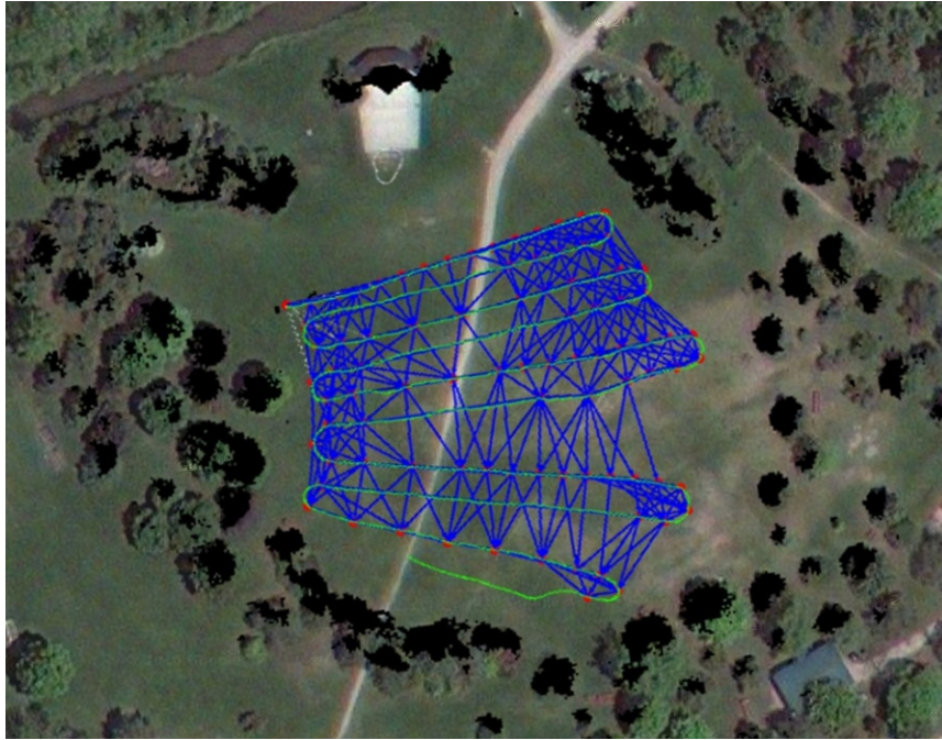
Figure 1.3: Highly connected pose graph and resulting map for scan registration based graph SLAM algorithm.
