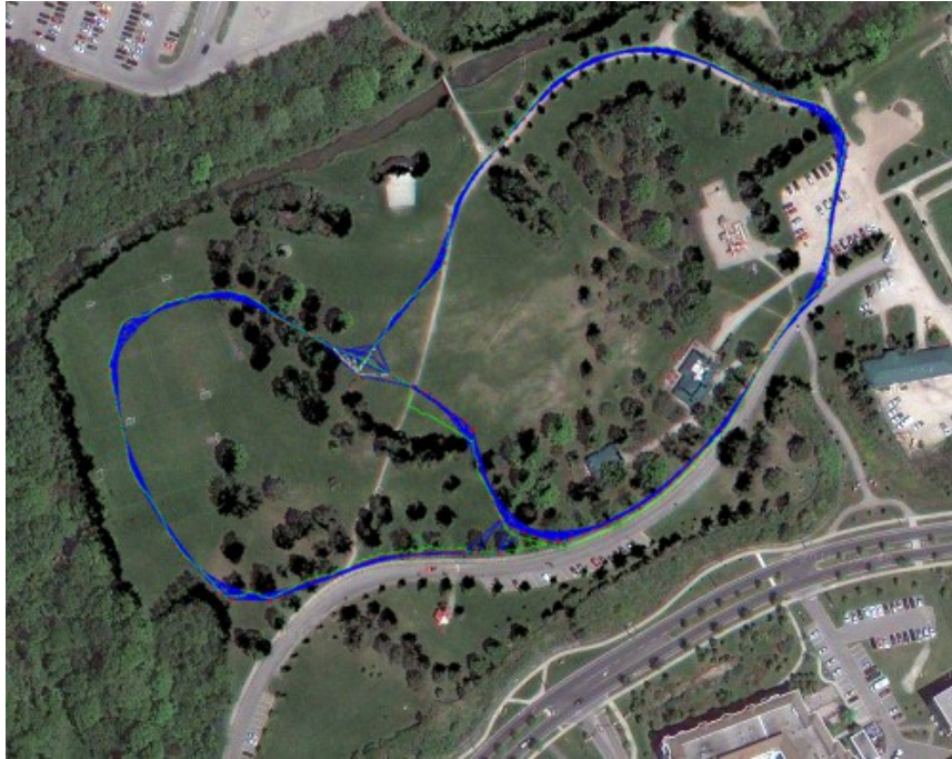
Figure 1.2: Reconstructed map and aerial image overlay for scan registration based graph SLAM algorithm.
