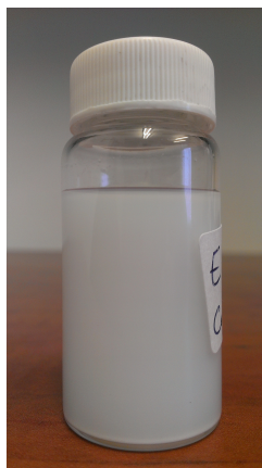
Figure 5.1: EC colloidal solution of \sim 15 g/L (1.5 wt.%) more than 9 months after the synthesis.
