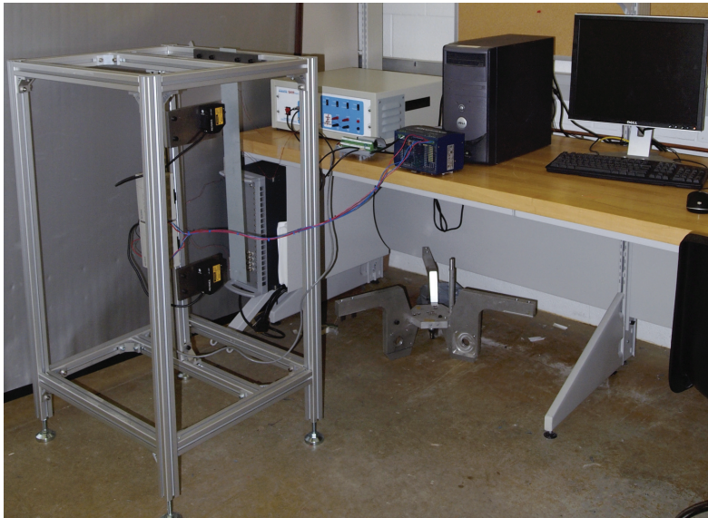
Figure 5.1: Experimental setup for vibration control and shape control of a steel cantilever beam
