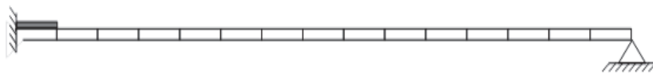
Figure 3.11: Optimal location of one actuator on a beam with pinned-fixed end conditions
