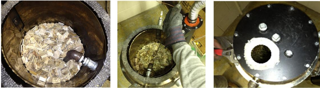
Figure 27: GEK IV reactor being filled with wood chips
