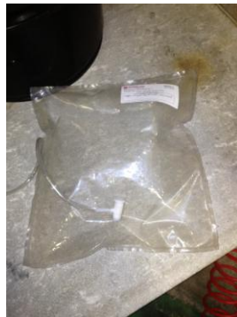
Figure 33: Gas sampling bag containing the collected syngas
