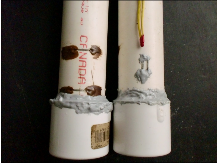
Figure 3.4: Location of thermistors of open water tests and example of different sizes and orientations of resistance sensors
