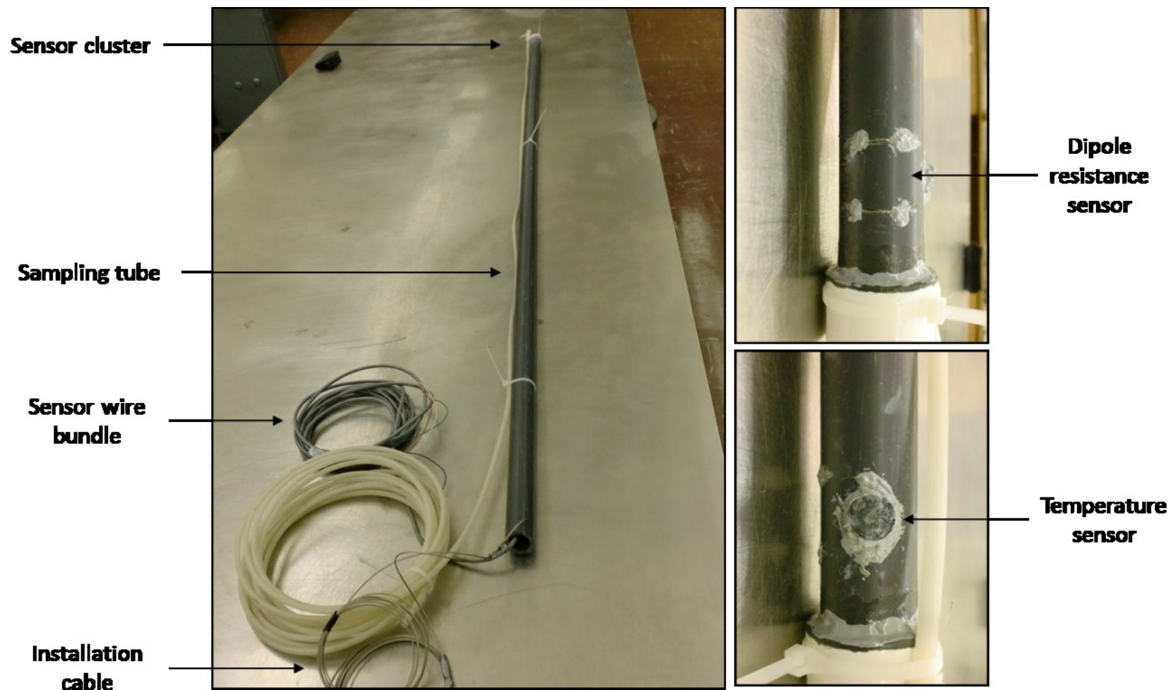
Figure 2.3: Field probe schematic. Temperature sensor shown was inserted in rubber stopper, which was force fit into the drilled hole. Other designs used temperature sensor fit directly in PVC. Sensors sealed with marine epoxy (LePage, Model 10-00397) and silicone (GE Model SE2184 24C).
