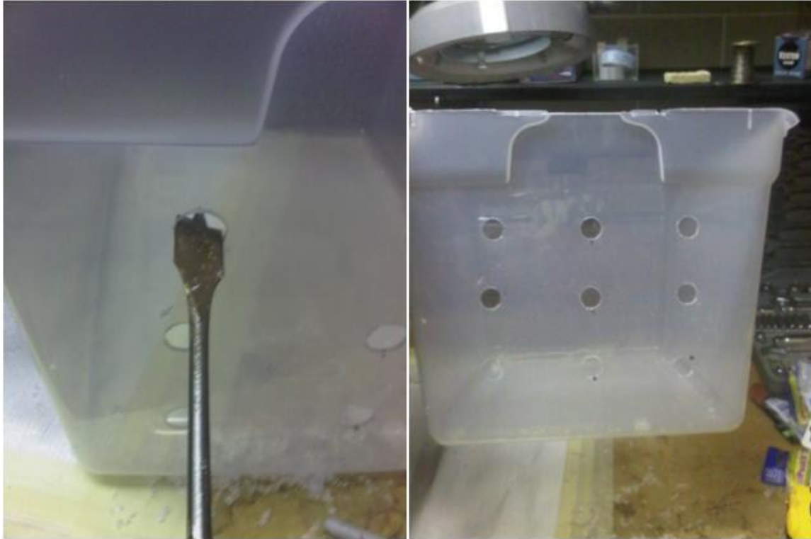
Figure D1: 9 holes (1.25 cm diameter) drilled in upstream end of main reservoir
