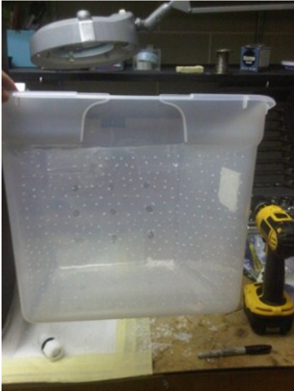
Figure D2: Approximately 400 1/16 inch holes drilled in downstream end of main reservoir
