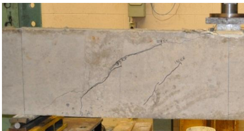
b) Low corrosion level beam D6-7.5%-UR
