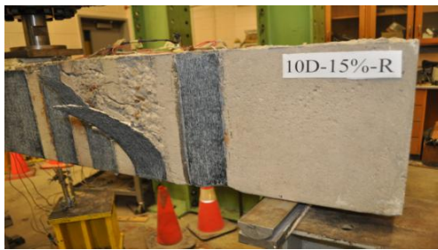
d) CFPR repaired beam 10M-15%-R
