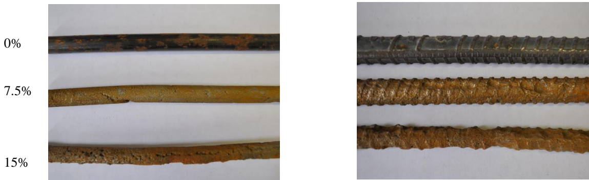
Figure 3.3 Photos of coupons of 10M and D12 ordered by corrosion level (0%, 7.5%, and 15%)
