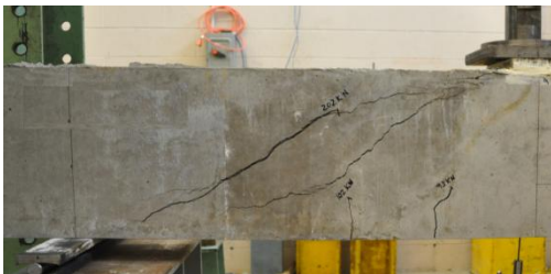
b) Low corrosion level beam D6-7.5%-UR-100
