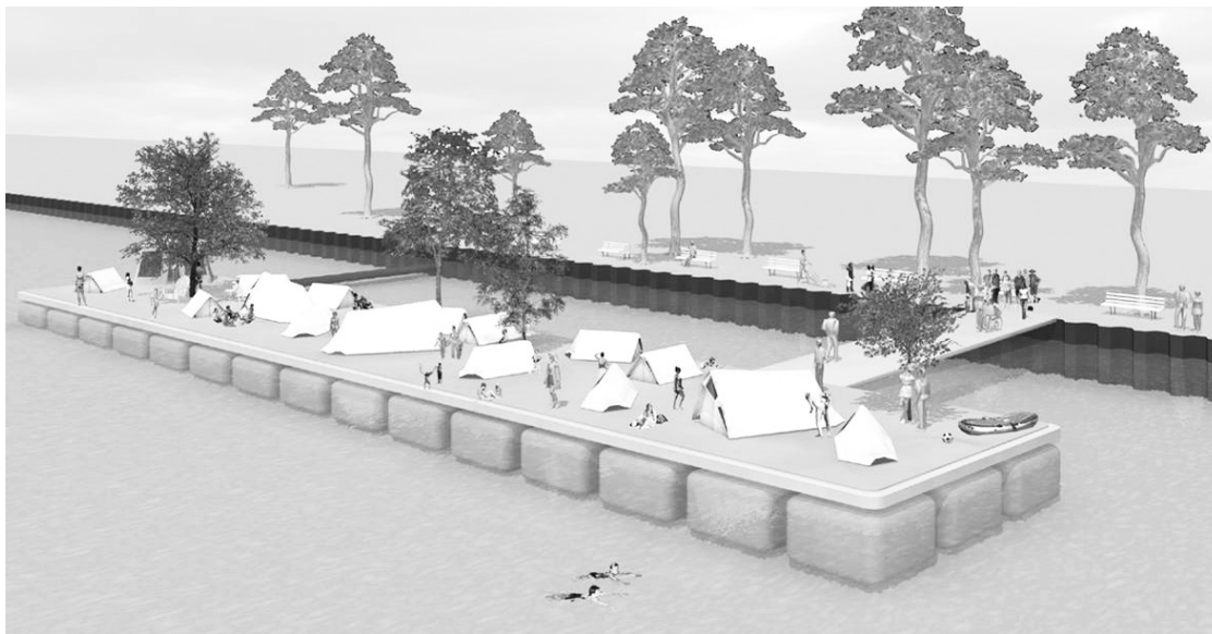
Fig. 3.12 A rendering of Raalf Steeg's Spree 2011 project demonstrates how the buoyant C.S.O. reservoirs double as a floating public dock that facilitates a variety of public activities at the water's edge.
