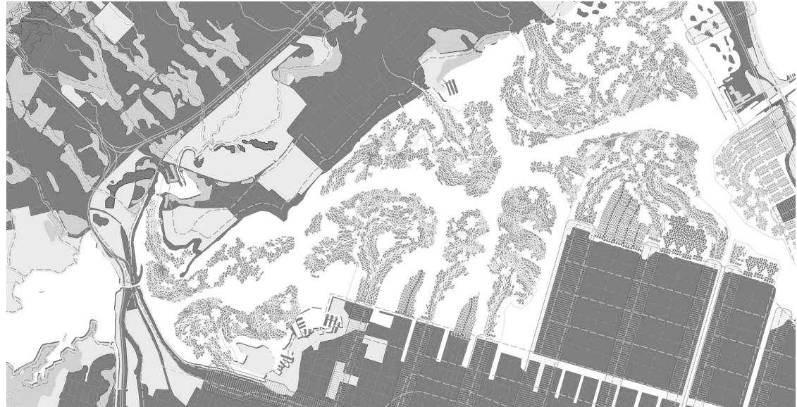
Fig. 3.3 A site plan of Jonah Humphrey's Landscape illustrates the deployment of buoyant, decentralized living machines in Hamilton Ontario's harbour. These clusters intercept sewer overflow by plugging into the city's existing sewer grid.
