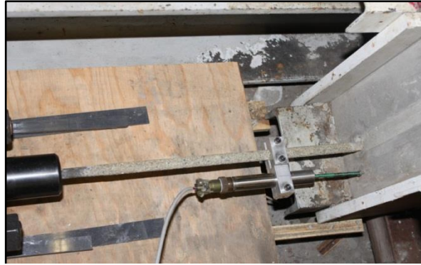
Figure 3.16 End slip measurement during prestress load release
