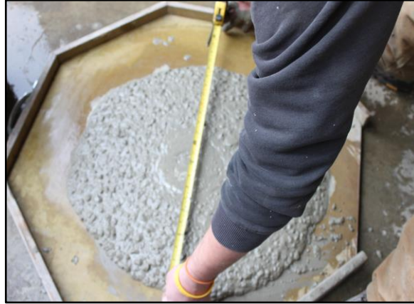
Figure 3.6 Slump flow measurement on SCC-mix3, VSI =0
