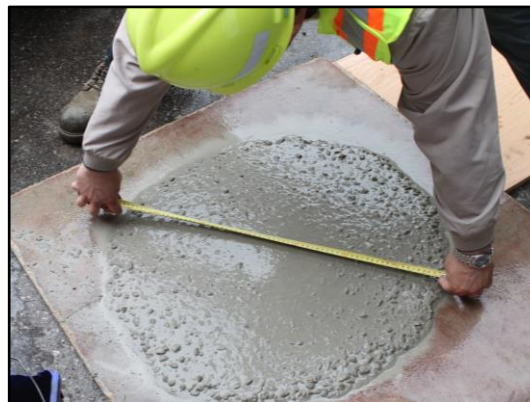
Figure 3.5 Slump flow measurement on SCC-mix2, VSI =1
