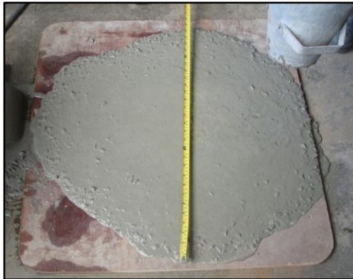
Figure 3.4 Slump flow measurement on SCC-mix1, VSI = 1.5
