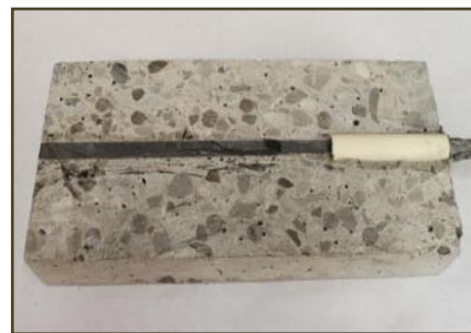
(d) Concrete slice showed the CFRP bar still in complete contact with concrete
