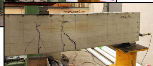
(c) Failure crack at the end of the shear span
