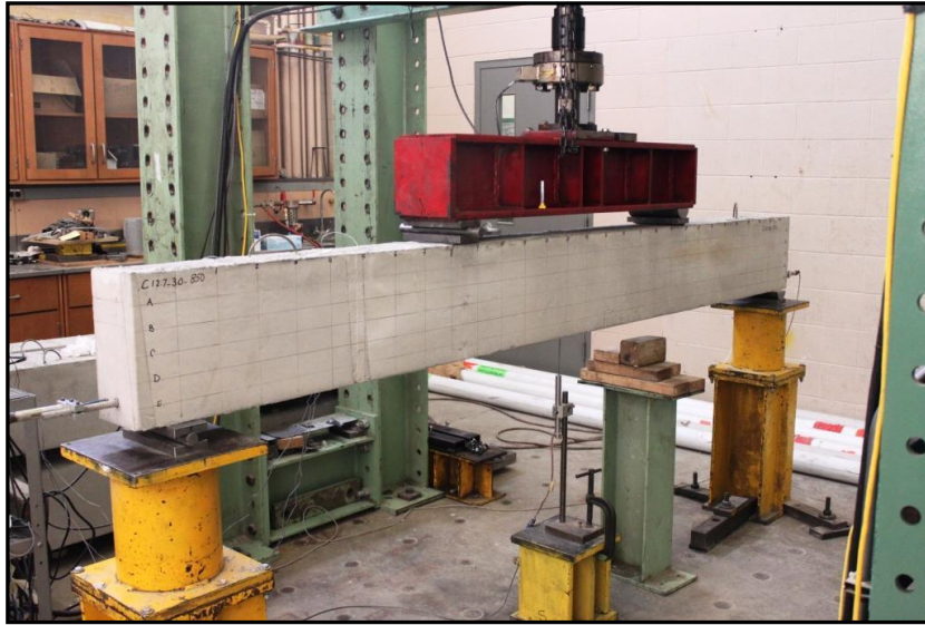
(a) Beam SC12.7-3.0-850 before flexural
