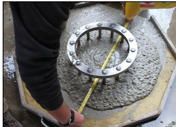
Figure 3.7 J-ring flow measurements on SCC-mix 3
