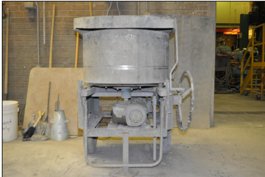
Figure 3.1 The pan-type revolving mixer
