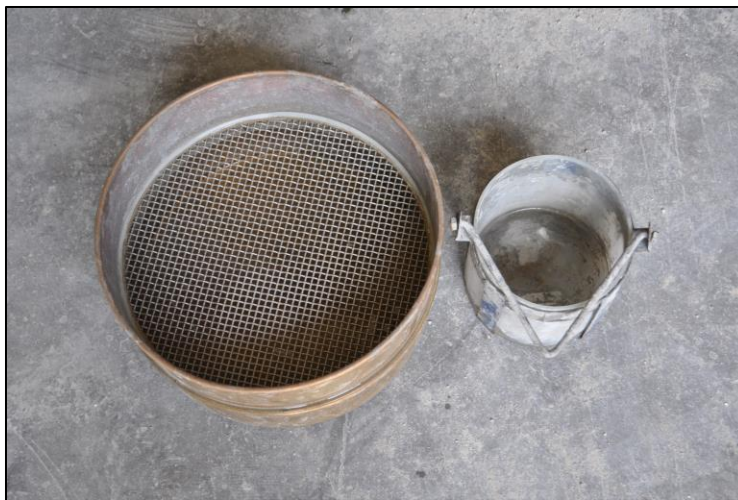
Figure 3.4 Sieve analysis apparatus for aggregate segregation
