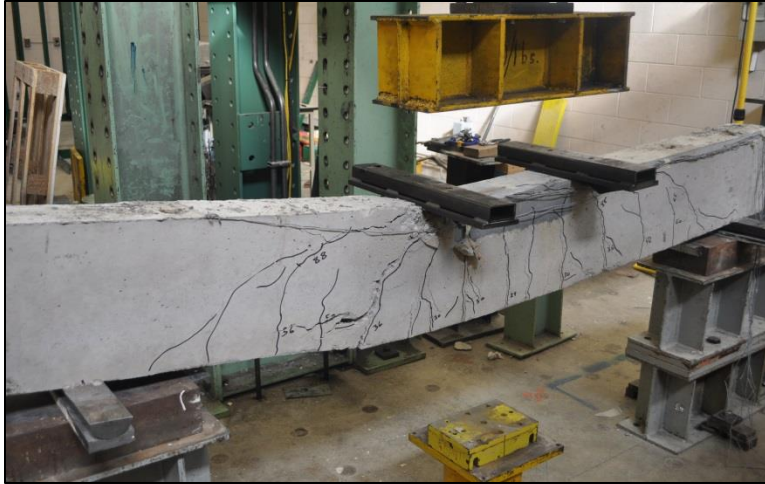
Figure 5.5 Failure mode for the top-patch repaired beam with Sikacrete-08 SCC
