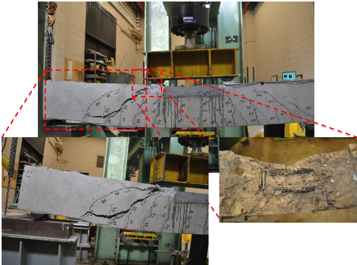
Figure 5.6 Failure mode for the top-patch repaired beam with mix M1 (SCC, no fibers)
