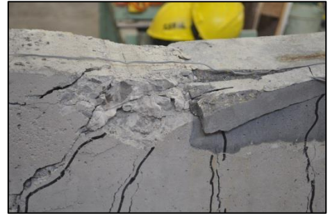
Figure 5.5 Failure mode for the top-patch repaired beam with Sikacrete-08 SCC
