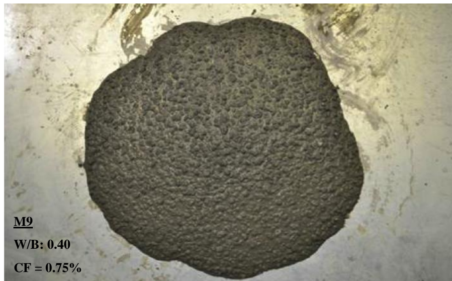
b) Mix M9: VSI = 0.5 (moderately stable); concrete shows very slight bleeding as a sheen on the surface and a very small mortar halo < 5 mm.
