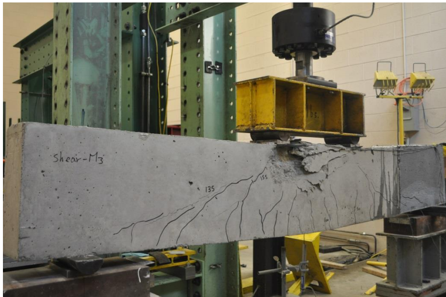
Figure 5.20 Failure mode of the shear-span repaired beam with mix M3 (CFRSCC, 0.50% fibers)
