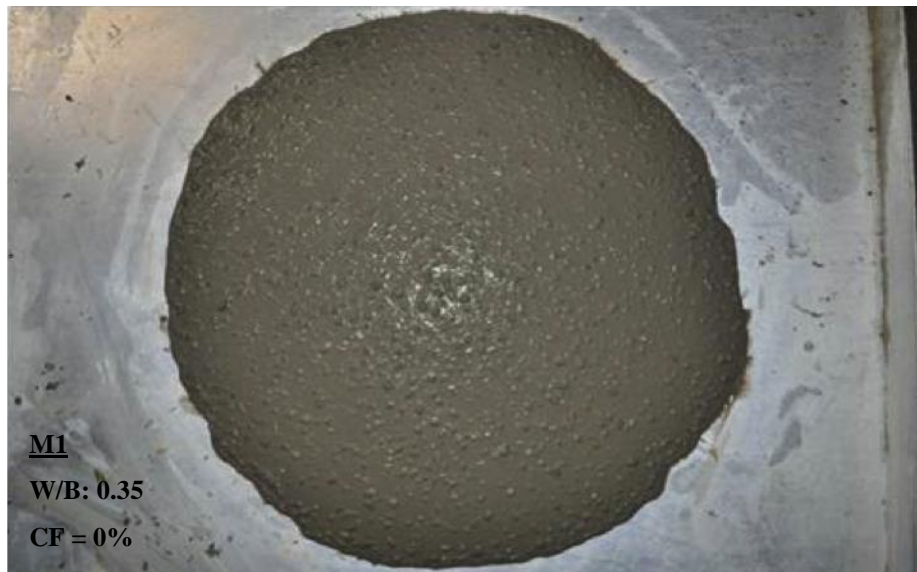
a) Mix M1: VSI = 0 (highly stable); no evidence of bleeding, mortar halo, and aggregate piling.
