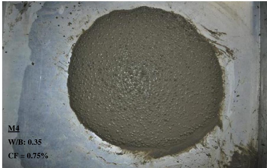
a) Mix M4: VSI = 0.5 (moderately stable); no evidence of bleeding but negligible coarse aggregate concentration at the middle of the flow patty and a very small mortar halo < 5 mm.
