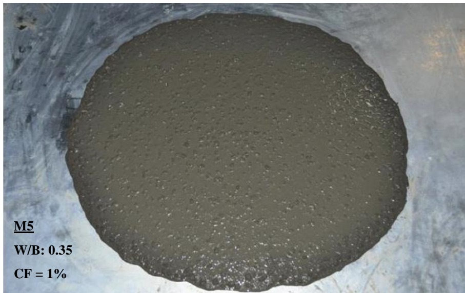
a) Mix M5: VSI = 0 (highly stable); no evidence of bleeding, mortar halo, and aggregate piling.
