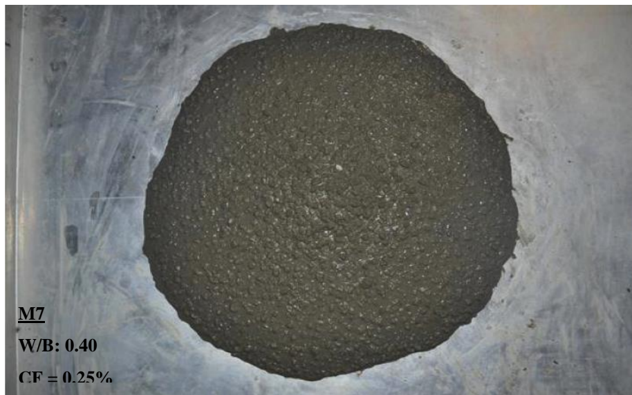
b) Mix M7: VSI = 0.5 (moderately stable); negligible coarse aggregate concentration at the middle of the flow patty and a very small mortar halo < 5 mm.
