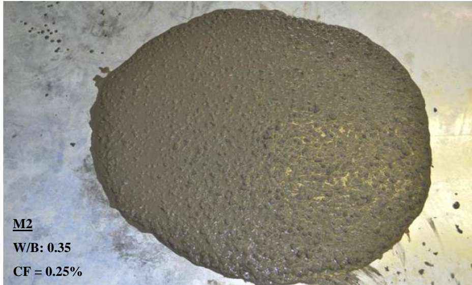
a) Mix M2: VSI = 0.5 (moderately stable); very slight bleeding and a very small mortar halo < 5 mm.
