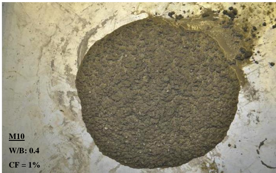
b) Mix M10: VSI = 1 (stable); concrete shows very slight bleeding as a sheen on the surface and a very small mortar halo < 10 mm.
