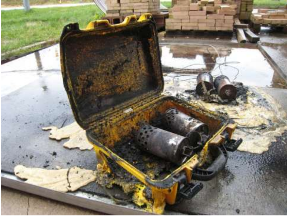
Figure 7-17. StatX FR Safe Storage Test Case after Unit Activation
