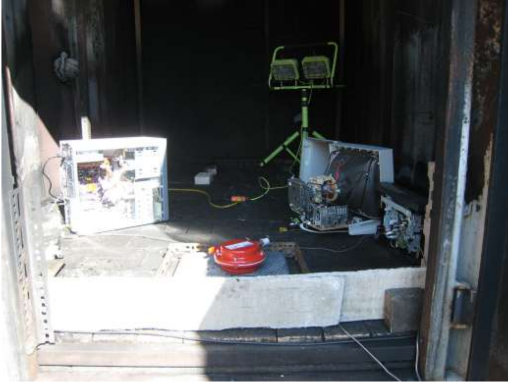
Figure 6-8. Electronics Exposure and Compartment Setup for DSPA 5-4 Agent Analysis Test
