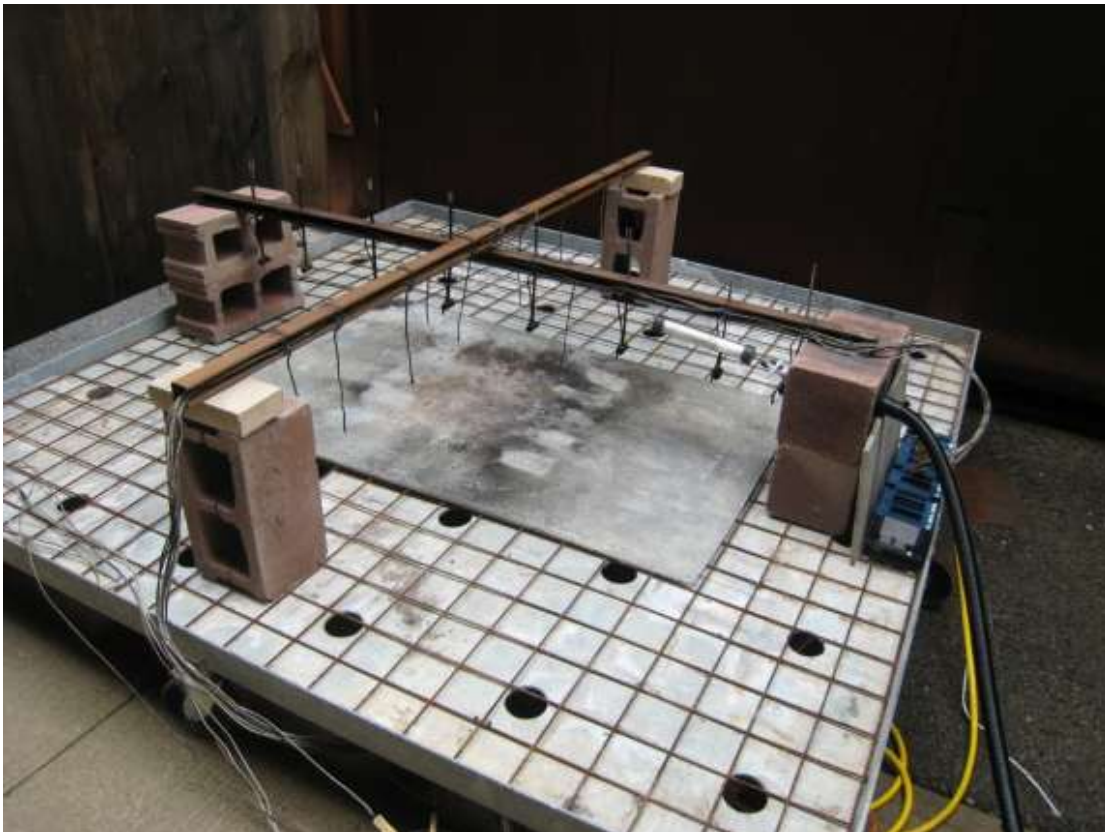
Figure 7-5. Safe Storage and Incendiary Potential Test Rig
