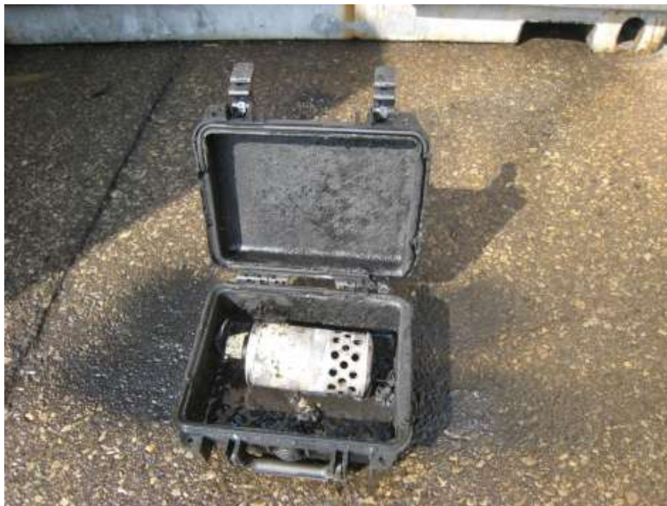
Figure 7-4. StatX FR Pelican Case Following Enclosed Unit Activation
