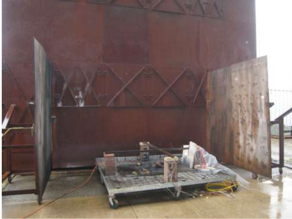
Figure 8-1. Incendiary Potential Test Setup and Ambient Conditions
