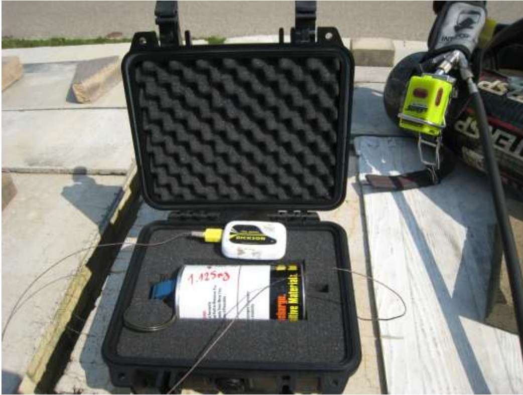
Figure 7-1. StatX Safe Storage Preliminary Test Rig
