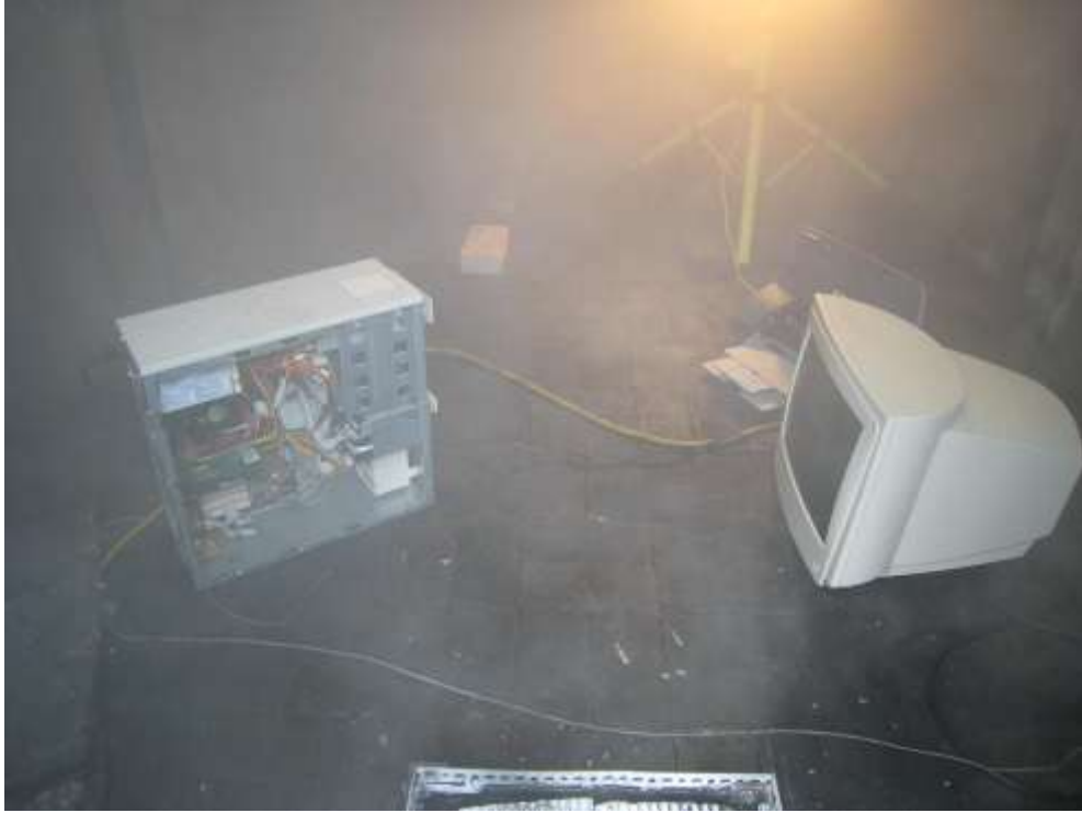
Figure 6-2. Electronics Exposure and Compartment Setup for StatX FR Agent Analysis Test
