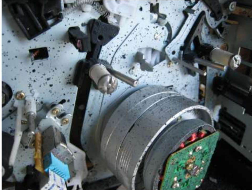
Figure 6-12. Slag Distribution on VCR from DSPA 5-4 Activation 60 cm Away
