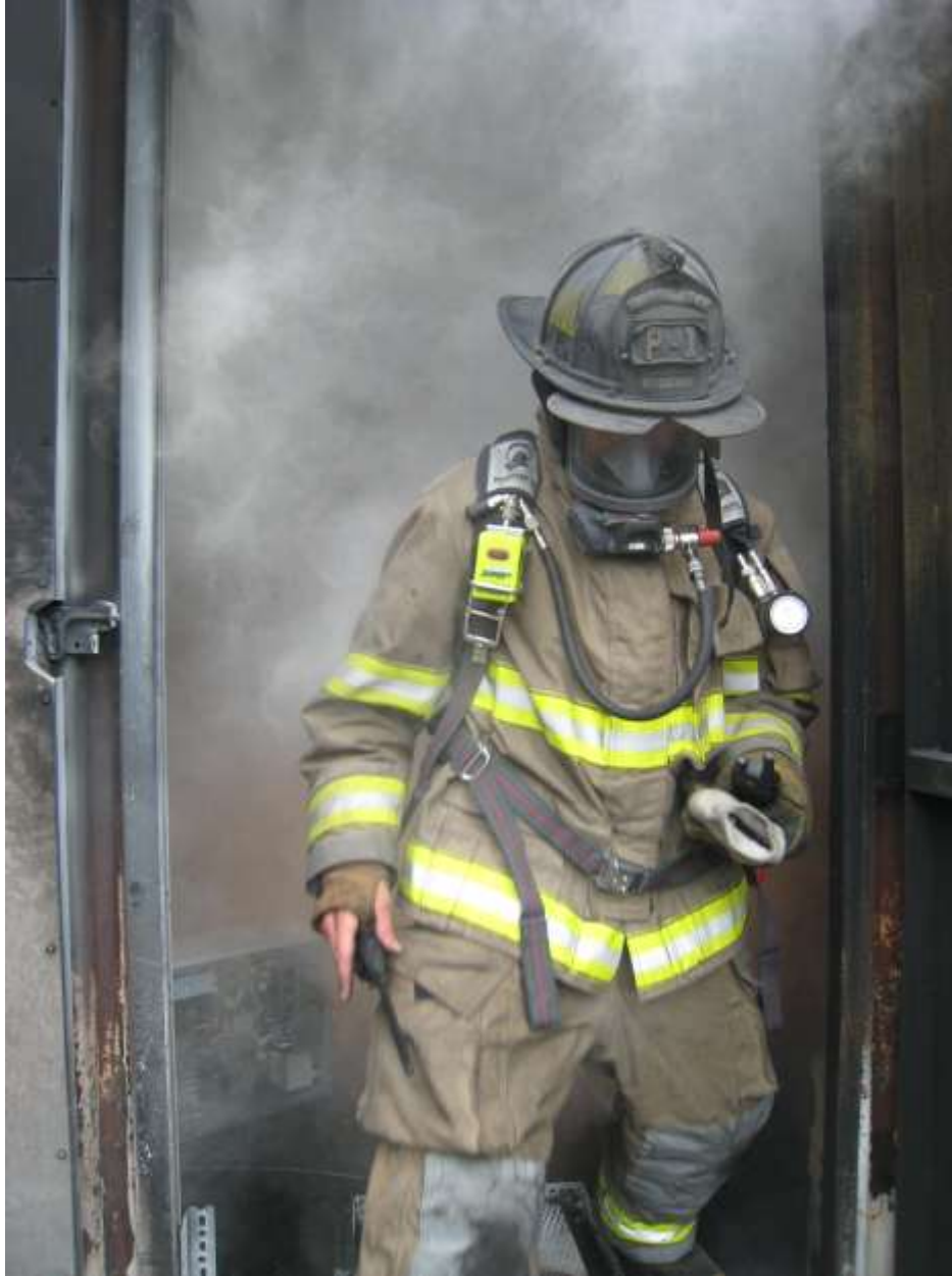
Figure 6-7. Aerosol Powder Collection on Firefighter Protective Ensemble and Breathing Apparatus
