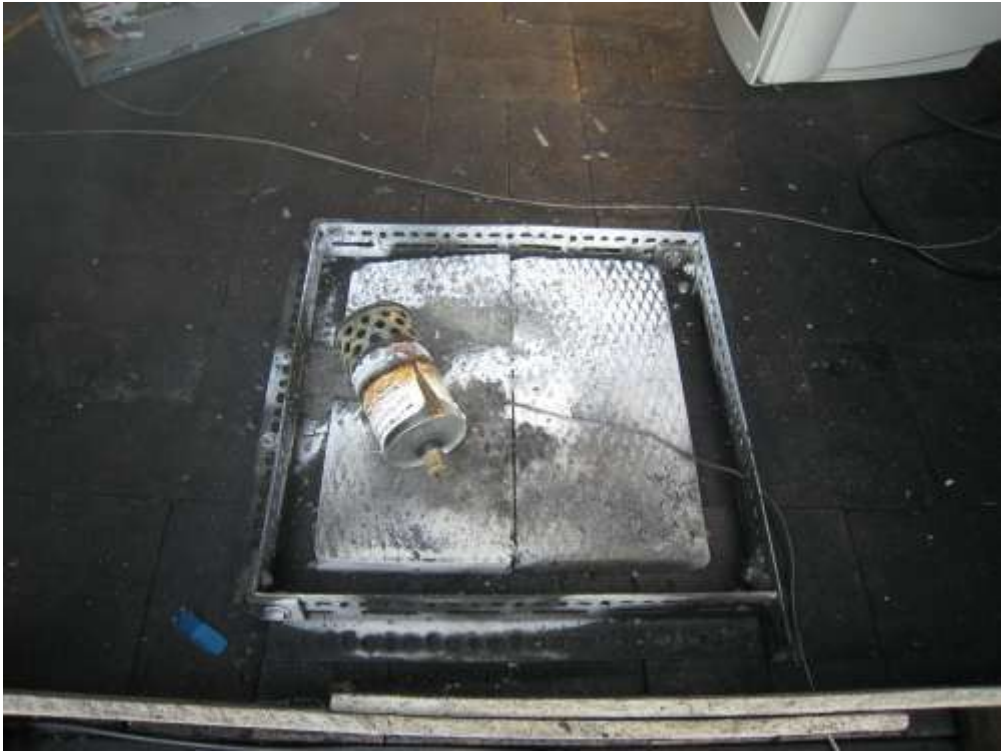
Figure 6-3. Location of Unit Activation for StatX FR Agent Analysis Test
