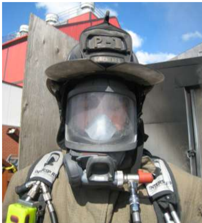
Figure 6-11. Aerosol Powder Collection on Firefighter Protective Ensemble and Breathing Apparatus
