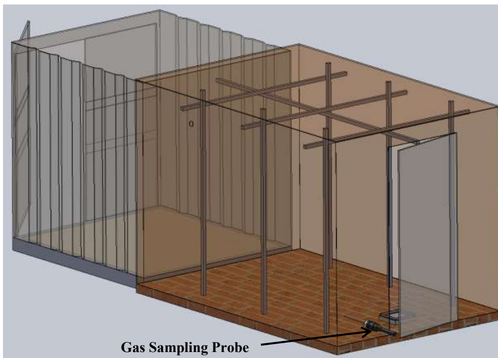
Figure 6-1. UW Shipping Container Burn Room Set-up for Test 5, Agent Analysis with Front Gas Sampling Position
