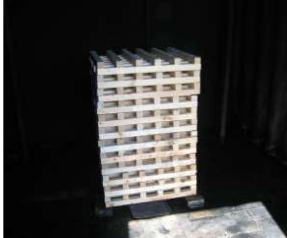
Figure 3-7. 4-Crib Softwood Fuel Load Configuration
