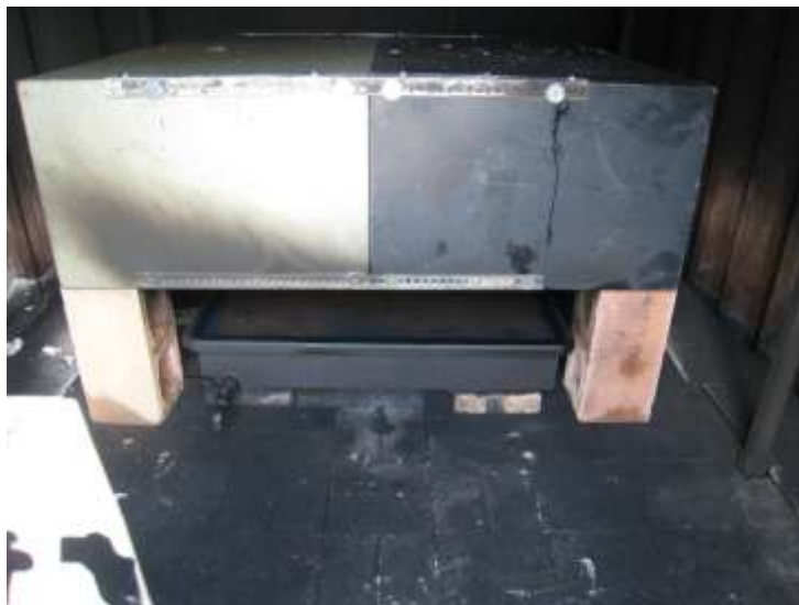
Figure 3-4. Mock Engine Enclosure used in Obstructed Diesel and Bilge Fire Suppression Tests
