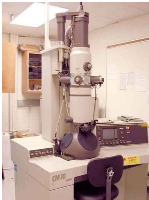
Figure 3.3 Philips CM10 TEM system
