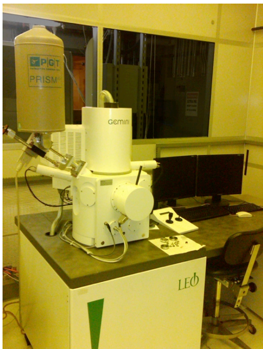
Figure 3.2 Leo FESEM SEM/EDS system
