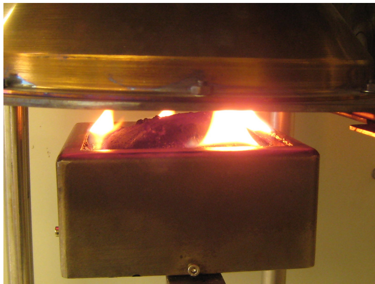
Figure 2.9: A burning specimen in the cone calorimeter test.
