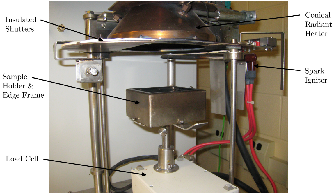
Figure 2.6: Detail of the specimen platform on the UWLFR cone calorimeter.
