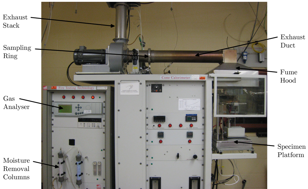
Figure 2.7: The UWLFR cone calorimeter, with relevant sections identified.
